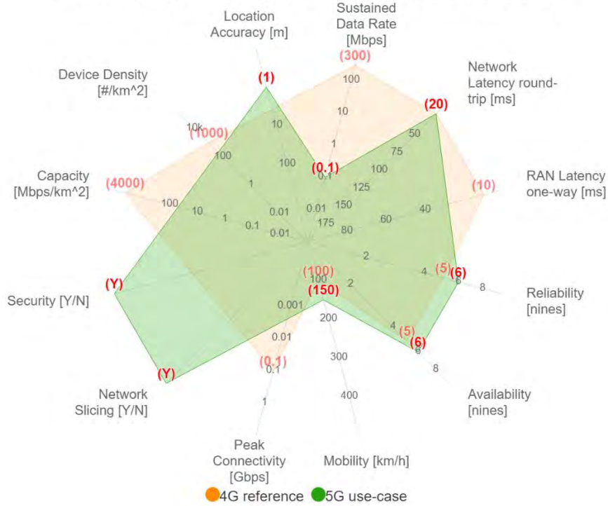
5G-VINNI UC1.1: Enhanced Mobile broadband under high speed mobility URLLC (Train operational services)
