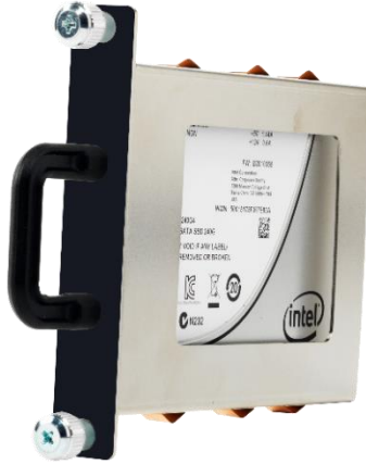
Figure 3. Removable SSD included with the M9537A
