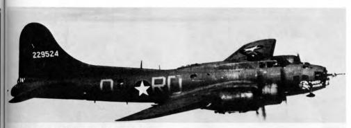
Note single machine gun protruding from nose.
