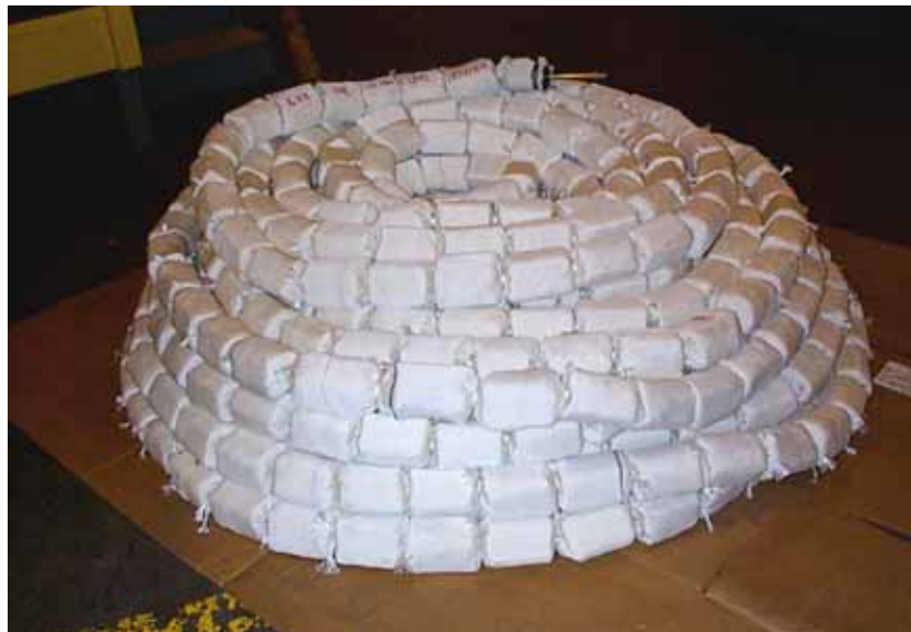
Charge, Demolition, HE Linear M58 Showing Blocks of C4 Explosive
