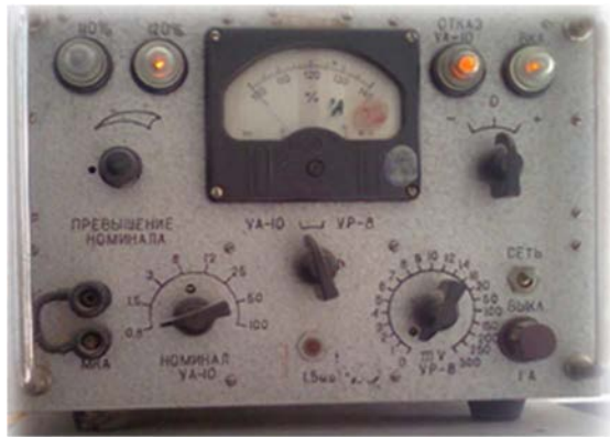
FIG. 2. Test device for prestart adjustment of emergency safety amplifiers made in 1956.
