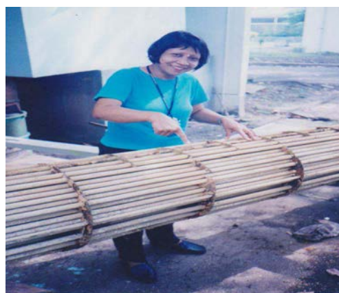
FIG. 6. Deterioration of baffle plates [5].
