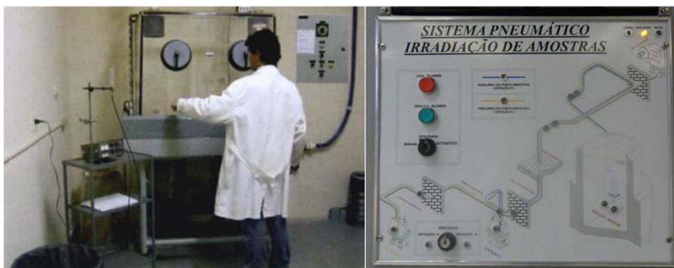
FIG. 2. Pneumatic irradiation system, user station (left) and control panel (right).
