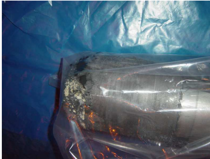
FIG. 8. The last 33 cm segment of the broken graphite plug.
