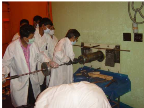
FIG. 7. Cutting operation by using auger.
