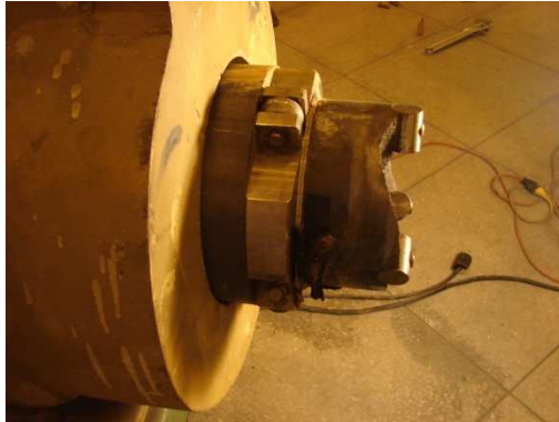
FIG. 3. Broken graphite plug (1 st break).
