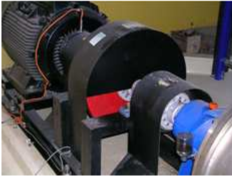
FIG. 8. New primary pump and inertia flywheel with online vibration monitoring system.
