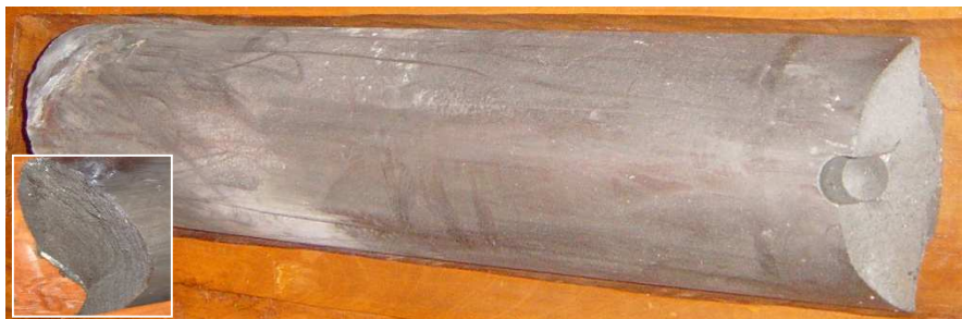
FIG. 5. Broken graphite plug (2 nd break).
