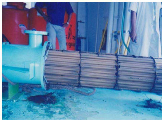
FIG. 4. Shell and tubes bundle of heat exchanger [5].
