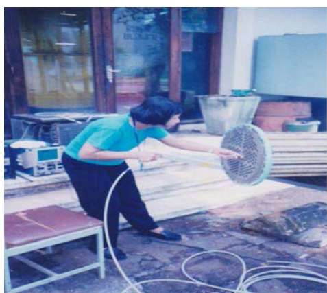
FIG. 5. Heat exchanger tubes inspection conducted in 2003 [5].
