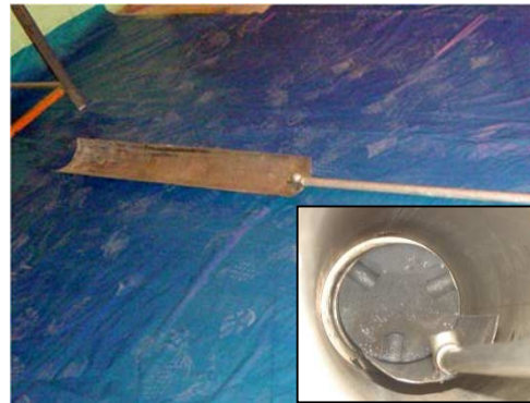
FIG. 4. Scoop used for BP plug removal.
