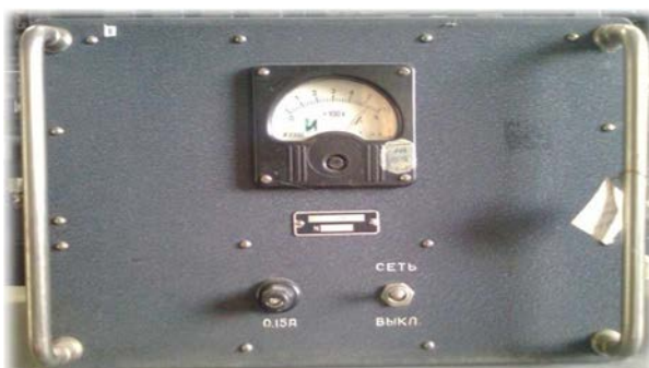
FIG. 1. Ionization chamber power unit made in 1966.
