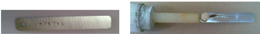
FIG. 5. Left) Carbon steel coupon before insertion; right) after insertion for a one-month period in the corrosion test rack in the cooling tower.
