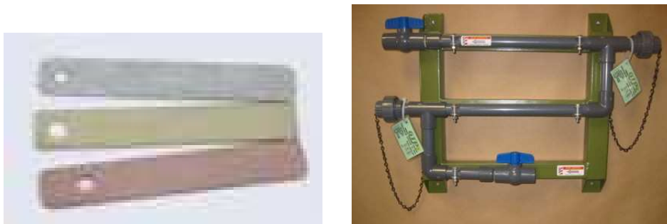
FIG. 4. Left) Coupons of different constructive materials; right) corrosion test rack.
