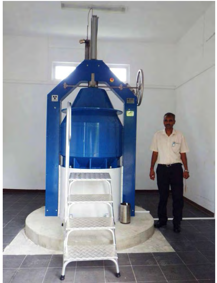
Ob-servo Ignis self-shielded cobalt-60 irradiator.
