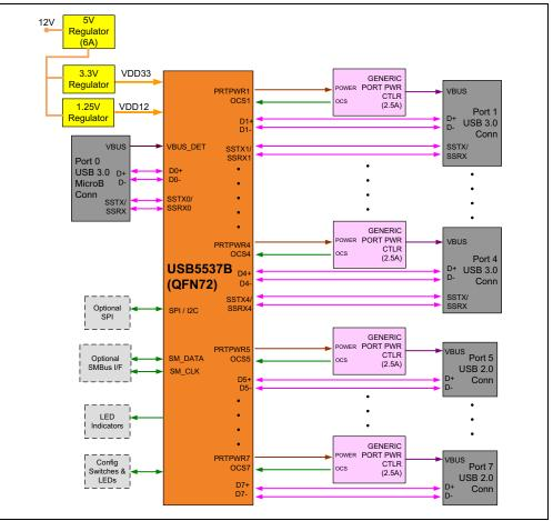
FIGURE 2-1: BLOCK DIAGRAM
