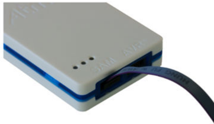
Figure 5-2. ATATMEL-ICE Debugger SAM Probe Connection
