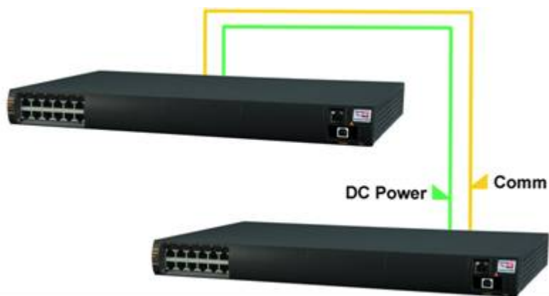
Figure 4-2. Secondary Midspan Power Backup
