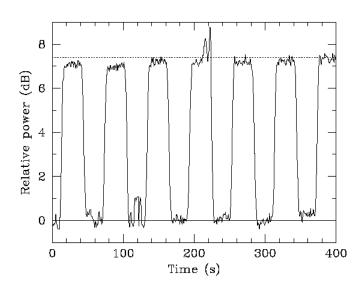
Fig. 5. – Measurements of Sun noise with a pair of 15LFA-JT Yagis. The dotted line represents the expected value for  $Y_{Sun}$  with 432 MHz solar flux S = 44 SFU and system noise temperature  $T_s = 119$  K.
