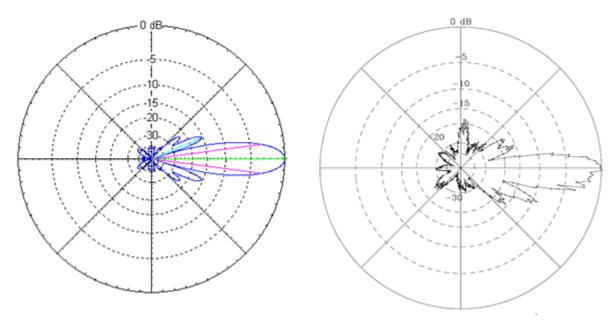
Fig 4. – Simulated (left) and measured (right) azimuth patterns of a pair of 15LFA-JT Yagis stacked horizontally, in horizontal polarization. The stacking distance was 1.2 m.
