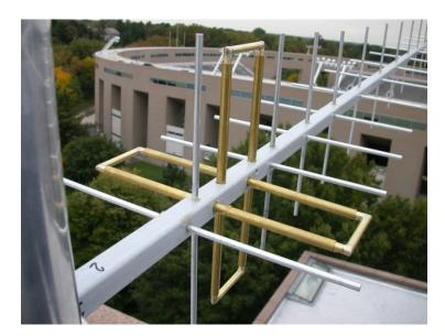
Fig. 3. – Rear view of a single Yagi showing construction details around the driven elements. The brass loops are fed at the center of their forward sides, inside the hollow boom. RG142 coaxial feedlines pass out to the rear. All elements are held in place with tight-fitting holes and a few drops of fiberglass resin.
