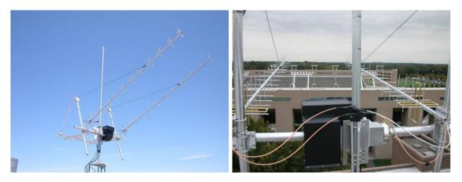
Fig 2. – A pair of 15LFA-JT rear-mounted Yagis on a simple mount with azimuth and elevation control. Separate feedlines carry signals for horizontal and vertical linear polarization from each Yagi to a power splitter. Light-duty dacron ropes serve as forward guys, to prevent boom sag.
