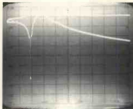
Fig. 6a) Second stage response, notch trace and low-pass trace 10dB/div.
