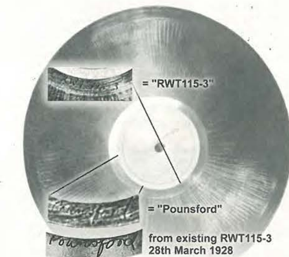
Fig. 5. Proof of the discs' ages comes from a photograph from July 1928 from which the signature "Miss Pounsford" and the serial number "RWT115-3" can be read. The current Phonovision disc dated 28 March 1928, bottom left, has identical markings.
