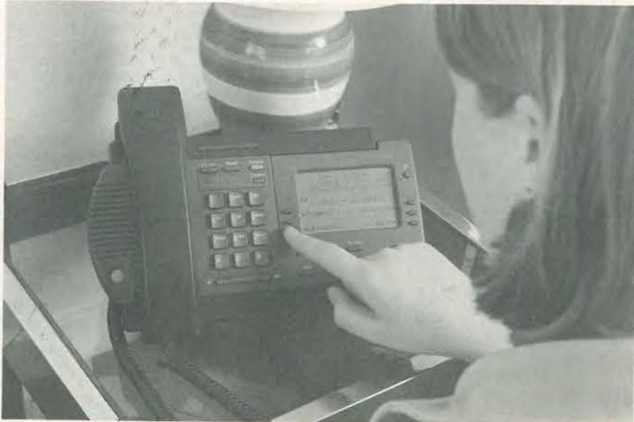
Phone banking... The Barclays Bank Screenphone gives customers access to banking details and other services without requiring a home computer. The ADSI protocol used specifies how voice and small bursts of data can simultaneously share the one analogue telephone line. The data transfer rate is 1.2kbit/s.
