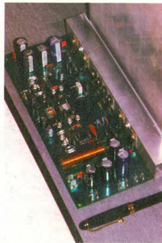
Giovanni's high-performance power amplifier mounted on its heat sink.
