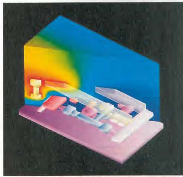
Raphael, a tool from Technology Modelling Associates, analyses the effects of parasitic interconnect in IC designs. When used with TMA Visual, the design can see the simulation results, in this case the electrical potential distribution in a static ram when the bit line is set to a higher voltage.
