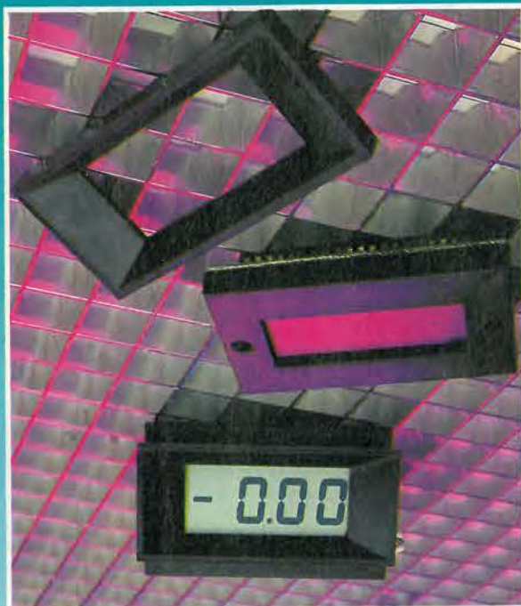
Incorporating the ICL7106 a-to-d converter, this digital panel meter has a full-scale input sensitivity of 200mV and a high input impedance of >100MΩ.
