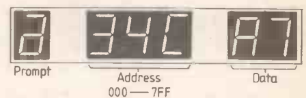
Fig. 1. A typical display. The 8086 processor has only 12 address lines, hence the hexadecimal address display consists of only three digits.
