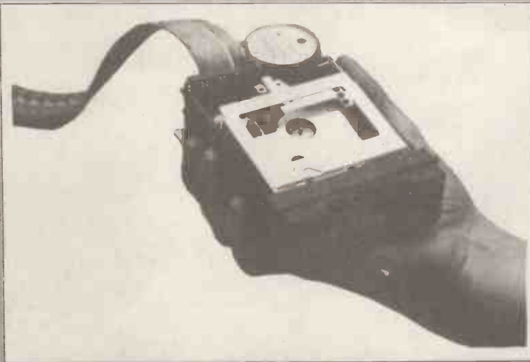
This micro-cassette drive comes from Hungary and is a low-cost alternative to many rivals. Each 2½-inch disc is housed in a rigid plastic cassette which offers some advantages in that it is better protected from the environment and can be provided with a solid core to improve the drive. It is claimed that the single-sided disc can hold up to 200Kbytes of data and can read or write its entire contents in less than a second. The bare drive costs £60 for one-off or is available in an applications kit with five discs, a head tuning disc, instructions and an interface cable for £100 (+v.a.t.). The UK agents are BATS-NCI Ltd, in London.
