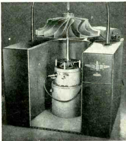
Ediswan portable gamma radiation monitor type 1030C, for indication of integrated dose up to 0.125 roentgens, and (right) de Havilland moving-coil vibrator for fatigue testing. Alternating thrust 250 lb and frequency range 0 to 1,000 c/s.
