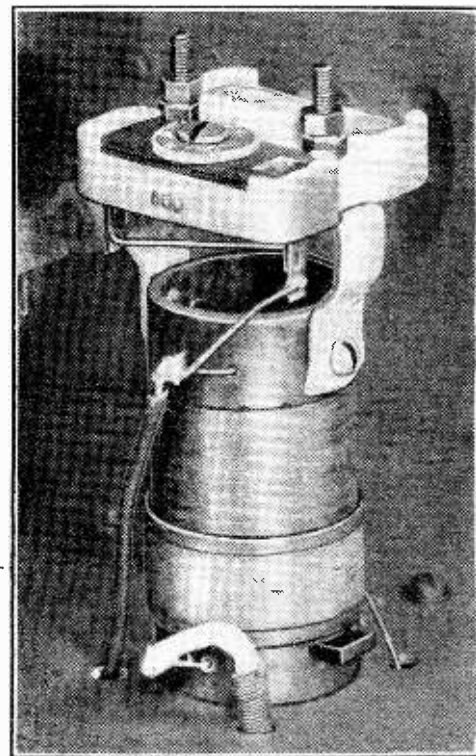
Constructional details of the IF transformer are given above, and on the right is shown the finished unit with the screening can removed.
