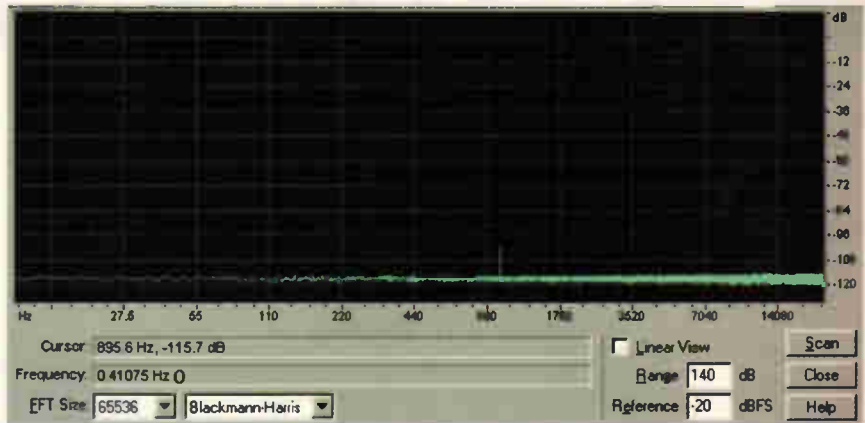
Fig 6 1003Hz at -120dB FS, captured using only 16 bits but correctly dithered and clearly visible above white noise in this FFT display. Note that the 'scan' function was used over 18s of audio to give a clearer representation of the true noise floor.
