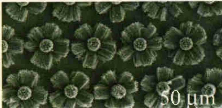
Workers at the Rensselaer Polytechnic Institute in the US claim to have achieved controlled nanotube growth, perpendicular to a prepared silica-coated substrate.
