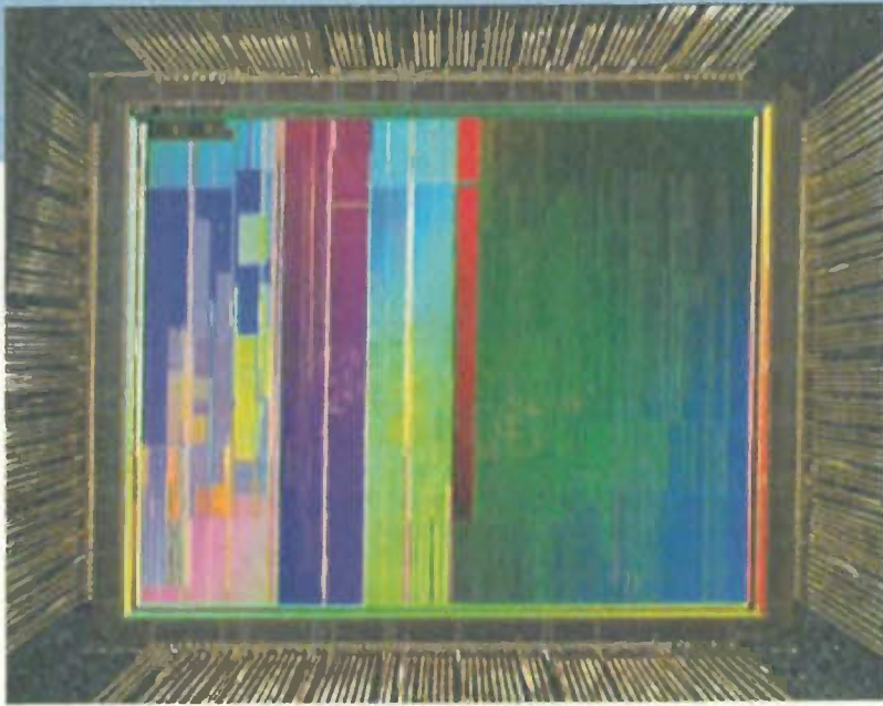
Alchemy is a name to be reckoned with in the chip design world, having its ancestry in the original StrongARM team. Its first chip, the Au1000 (above), is back from the fab and undergoing testing. Like Xscale, clock frequency and hence power can be dynamically scaled. Initial figures indicate that running at 1.25V and 200MHz, the chip dissipates 200mW, while at 1.5V and 400MHz power is up to 500mW.
