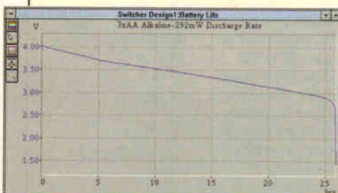
Fig. A. Typical plot of battery life, using the Micropower SwitcherCAD software, shows battery voltage by time with a 292mW load.
