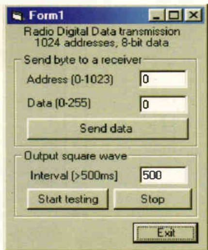
Fig. 15. User screen of the demonstration software, which allows you to send an 8-bit data word to a receiver specified by the address. If the 'Start testing' button is clicked, a square wave signal will be produced at the outputs of the specified receiver unit. The periods of logic high and low are determined by the value of 'Interval'.
