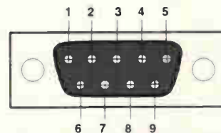
(a) 9-pin male socket viewed from the back of the computer
