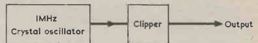
Fig. 1. A simple crystal calibrator offering an output at 1MHz and its harmonics
