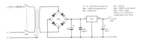
Figure 2: Circuit diagram of display unit.
