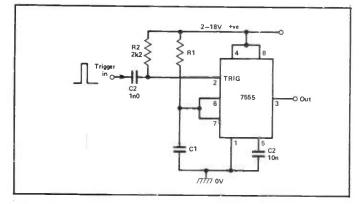
Figure 20: Simple electronically-triggered 7555 monostable.
