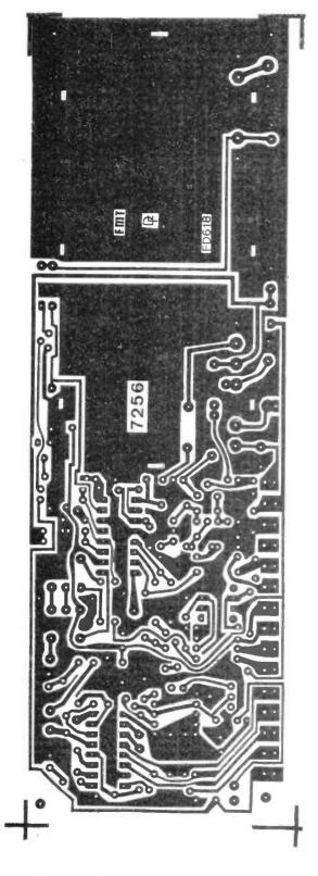
Figure 2b: PCB pattern for the underside.
