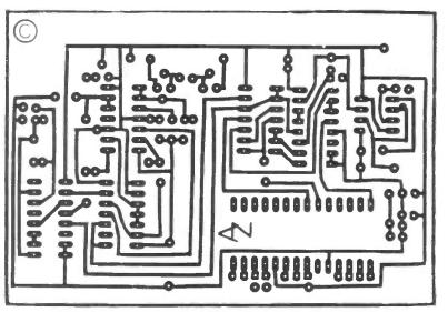
Figure 1: PCB foil pattern for main board of the Digital Capacitance Meter (July '83).
