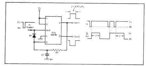
Figure 18: Retriggerable JK-type monostable.
