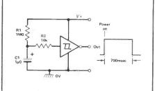
Figure 9: 'Noiseless' push-button switch.
