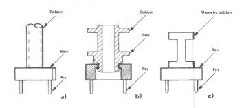
Figure 1: Bobbin — base structures. a) Bobbin and base in one unit; b) Separate bobbin and base — bobbin snapped into place; c) Bobbin bonded to the base.
