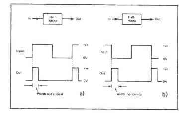
Figure 1: A 'half-mono' circuit may be used to detect a) the leading or b) the trailing edge of an input waveform.
