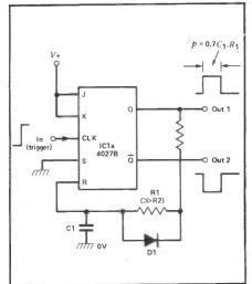
Figure 16: JK-type flip-flop used as a
