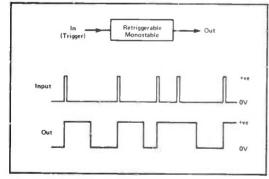
Figure 4: A retriggerable monostarts a new timing cycle on the arrival of each new trigger signal.
