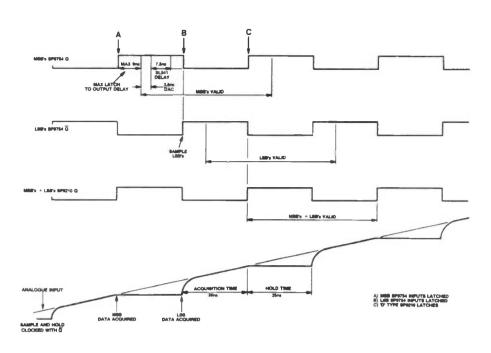
Figure 3: Timing diagram for the 20MHz clock.
