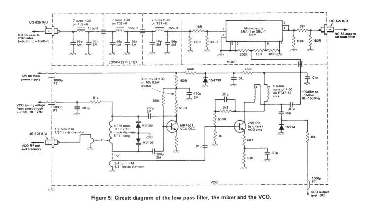
The VCO consists of an MRF901 Colpitts oscillator (a *BF240* would be an adequate European substitute) coupled to a wideband 2N5179 (*BFR91*) amplifier. The MRF901 was ultimately chosen for the oscillator transistor because of its well-behaved phase-shift characteristics between 90MHz and 150MHz. The two MV109 (*TOKO KV1210*) hyper-abrupt Epicap diodes act as tuning capacitors and account for the oscillator's wide tuning range.
