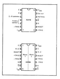
Figure 22: Outlines and pin notations of the 4047B monostable/ astable IC and the 4098B dual monostable.
