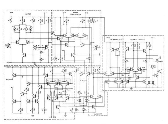
Figure 3: Circuit diagram for the NE564, with errors corrected (see text).
