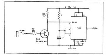
Figure 21: Pulse-triggered 7555 monostable.
