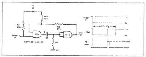
Figure 14: Resettable NAND-type monostable.
