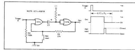
Figure 13: Resettable NOR-type monostable.
