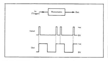
Figure 2: A standard monostable generates an accurate output pulse on the arrival of a suitable trigger signal.
