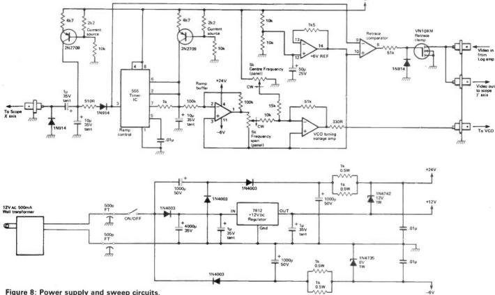
Figure 8: Power supply and sweep circuits.
