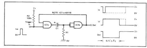
Figure 12: 2-gate NAND monostable is triggered by a negative-going signal and generates a negative-going output pulse.
