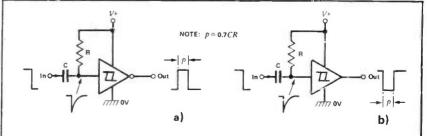
Figure 8: Trailing-edge detector circuits giving a) positive and b) negative output pulses.
