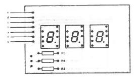
Figure 6: Component overlay for display unit.
