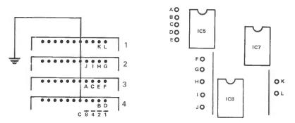
Figure 6: Connections to thumbwheel switches for the 720 Channel Airband Receiver.
