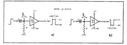
Figure 7: Leading-edge detector circuits giving a) positive and b) negative output pulses.
