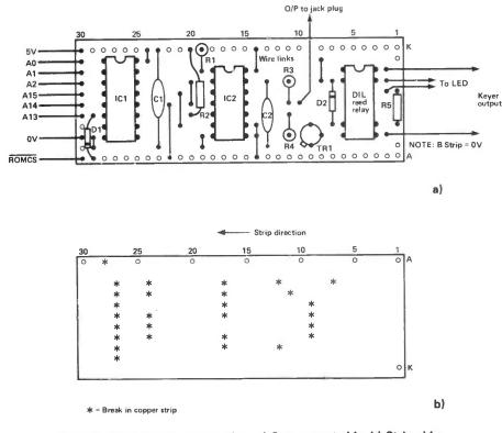
Figure 3: Strip board construction. a) Component side. b) Strip side.
