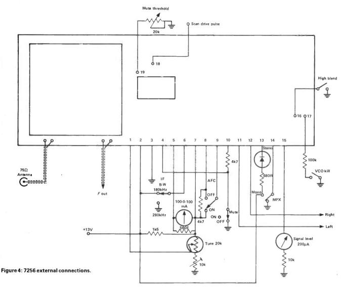
Maximum resistance corresponds to most sensitive mute operation. 5. The VCO in the stereo decoder is set by simply tuning to a known stereo transmission, and adjusting RV2 until the LED lights. If it doesn't, then make sure you've connected the LED the right way round before looking for anything more subtle.
