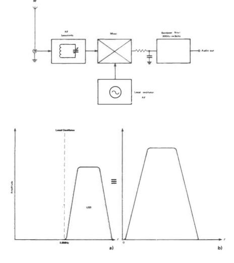
Figure 1: Direct conversion basics a) USB signal with RF injected locally to set the datum point for the resultant audio spectrum. b) The resultant audio spectrum.
