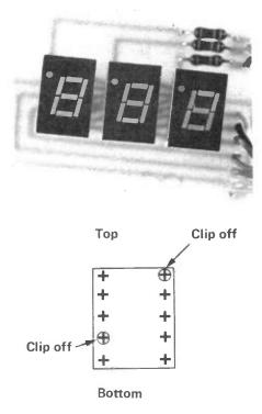
Figure 7: Trimming details for displays.
