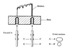
Figure 3: Pin insertion.
