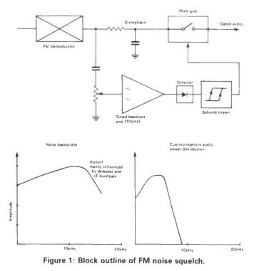
occupies a broad spectrum, with substantial energy at high audio frequencies. It will be tailored to a certain extent by IF filtering, but not so significantly as to prevent the use of a tuned audio filter above the audio bandwidth to amplify and detect the signal to be used for muting the audio output. The block outline of FM noise squelch is shown in *Figure 1*.
