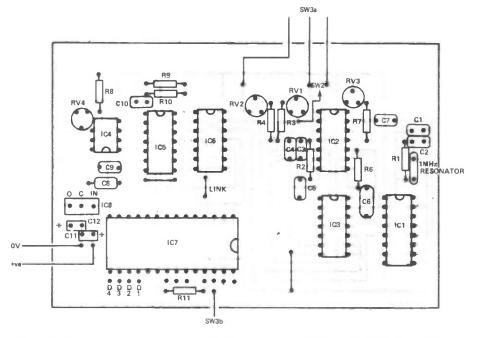
Figure 2: Note the change to the overlay in the region of IC5 of the DCM (July '83).
