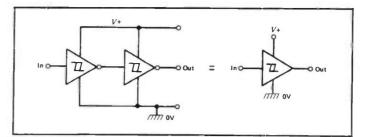
Figure 6: A non-inverting Schmitt can be made by wiring two inverting Schmitt elements in series.
