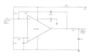
Figure 3: The CA3130 op-amp configured as an integrating filter,
