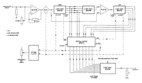
Figure 1: Block diagram for the SP9000 series-based A/D convertor.
