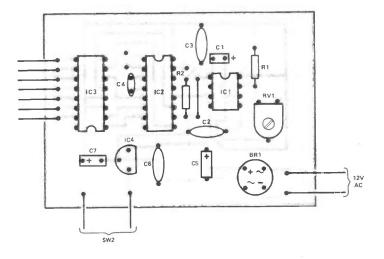
Figure 4: Component overlay for timer unit.
