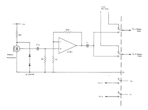
inserting its signal via a switch to the channel faders is quite sufficient here and the circuit diagram for this is shown in *Figure 2*. Note: As there is always the possibility of breakthrough, the supply to the pre-amplifier should be broken by the switch when slating is not required.
