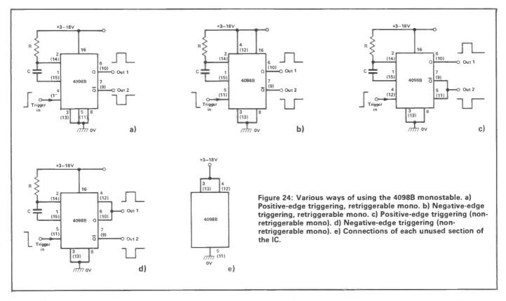
*Figure 24* shows a variety of ways of using the 4098B. Note that in these diagrams the bracketed numbers relate to the pin connections of mono 2, and the plain numbers to mono 1, and that the RESET terminal is shown disabled (pin 3 or 13).
