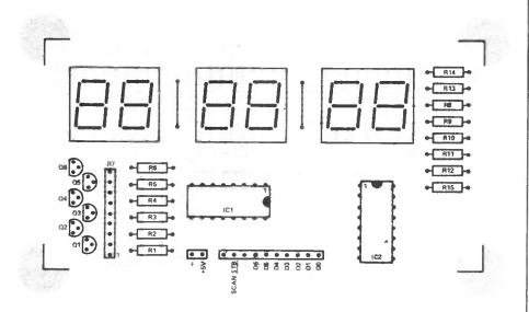
Figure 7: Overlay for updated version of the Rewbichron II display (April '83, May '83).
