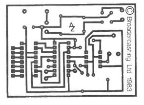
Figure 3: PCB for timer unit.
