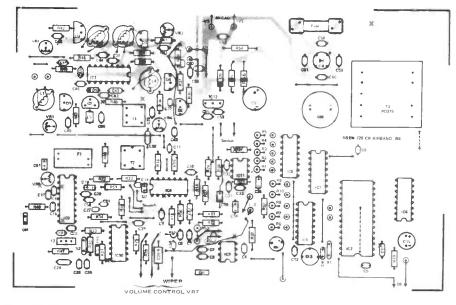
Figure 5: Component overlay for the 720 Channel Airband Receiver showing positions through board links in blue (Sept '82, Oct '82).
