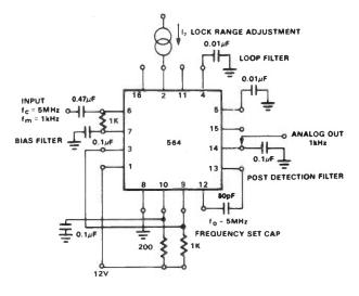
Figure 5: Circuit for an FSK decoder that incorporates an NE564.
