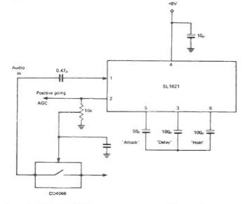
Figure 3: SL1621C AGC generator also controlling mute in an audio-derived application.
