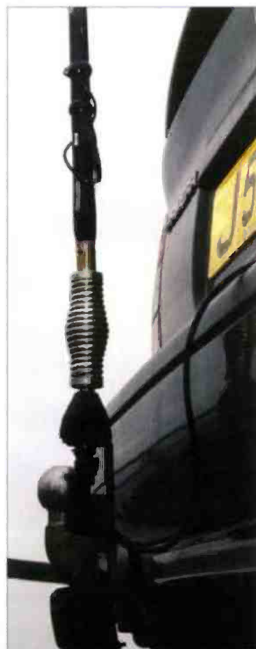
Fig 2: This picture shows the heavy duty, tight wound, chrome design mounting spring sent with the Highlander for review and is mounted between the base of the antenna and the feed point.
