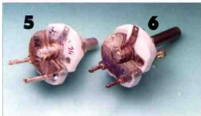
Fig. 5: The photograph shows two single variable capacitors, Type 5 (left) of 10pF and Type 6 of 25pF both are suitable for use as antenna trimmers, etc.
