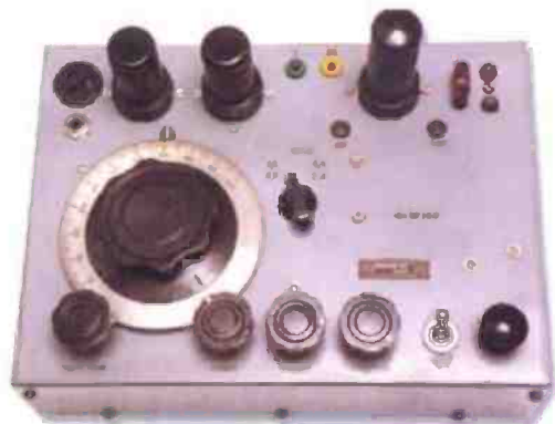
Fig. 3: The British-made 'Para' set copy, shown with two receive valves (top left), single transmit valve (top right). The miniature Morse key is shown on the lower right (see text).
