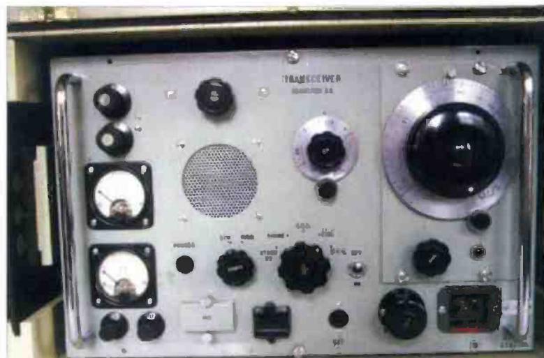
Fig. 1: The strange 'marine' set, with its unknown 'SSD' and 'FIRE' option on the centre mode switch (see text).
