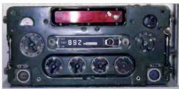
Fig. 5: The Chinese 892 set, showing the read-out tubes along the top with switch frequency selection along the bottom (see text).
