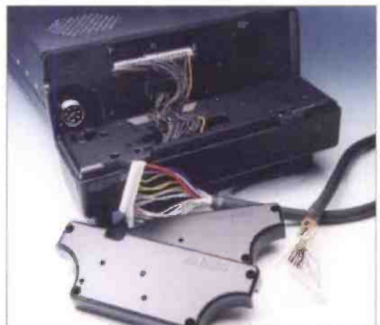
Fig. 2: The Alinco DX-70 (details same for the DX-70 and TH models) front panel detached, illustrating cable connections. The cable cover boxes (lower centre) are secured over the cable entry-exit points and are secured by (supplied) screws. The (front panel) cover box also provides a good mounting point for various methods of attaching the unit operationally (see text).
