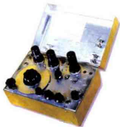
Fig. 4: The French reproduction 'Para' set. This version is complete with lid and frequency chart and valve retaining clips (see text).
