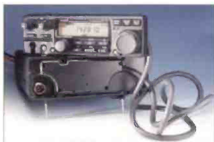
Fig. 1: The EDS-4 1.5m front panel remote control cable kit shown as fitted to an Alinco DX-70TH. (See text for comments on the microphone socket).
