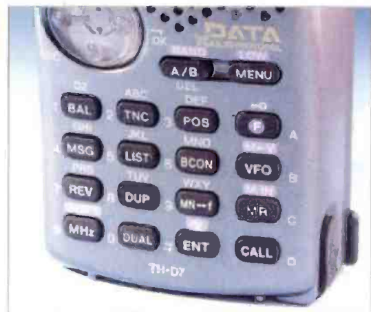
Fig. 1: Most controls are 'dual function'.
