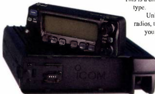
The detachable front facility of the IC-207H which G0RSN found to be very easy to use.
