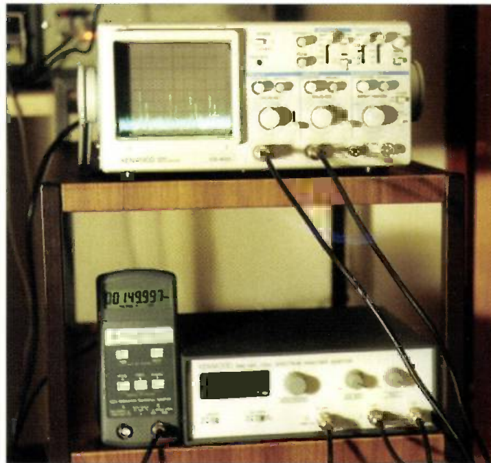
Fig. 5: The Kenwood trio set up in the lab for test, showing the counter reading 149.993MHz.
