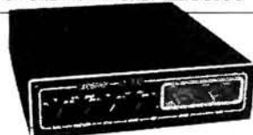
VHF POWER AMP.
