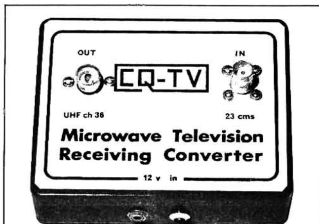
Probably the simplest of the commercial devices the CQ Centre receiving converter will allow initial ATV experiments to be made at 1.3GHz
