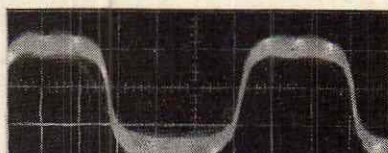
Fig. 9: Signal at the output of the pulse clipper stage shown in Fig. 7.
