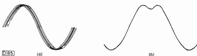
Fig. 2: Faulty (a) and correct (b) convergence coil drive waveforms, Sony Model KV27XRTU.
