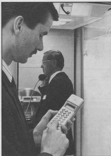
Digital Telepoint CT-2 handset made by Siemens and due to enter full service in 1991.
