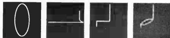
Capacitor 33uF Transistor E-C Transistor B-E B-E 1uF + 68ohms
