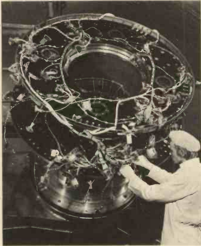
Geos. The Geos structure is seen during the installation of the wiring harness. The thrust-tube and platform structure can be clearly seen. The apogee boost motor is placed inside the thrust-tube. (By courtesy of British Aerospace)
