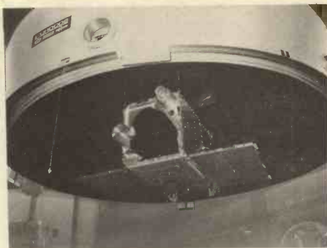
TD-1A. A structural model of the 472kg TD-1A spacecraft in position prior to space simulation tests. TD-1A was launched in 1972 into a 540km orbit, inclination 98 degrees, and was an ultra-violet astronomy satellite. It was 3-axis controlled and had a box-type structure. The only deployed appendages were the solar arrays which were flat panels. (By courtesy of European Space Agency)
