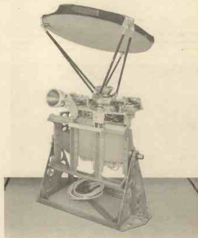
SMMR. Scanning Multichannel Microwave Radiometer, flown on the Seasat and Nimbus 7 satellites. The offset paraboloid antenna is 70cm across, and scans 25 degrees each side, driven by the mechanism which is visible. The central microwave horn is a very advanced 5-frequency device, and three calibration horns are also visible. The electronics are housed in the three bays beneath. Note the 12 inch ruler attached to the ground handling support. (By courtesy of Jet Propulsion Laboratories)
