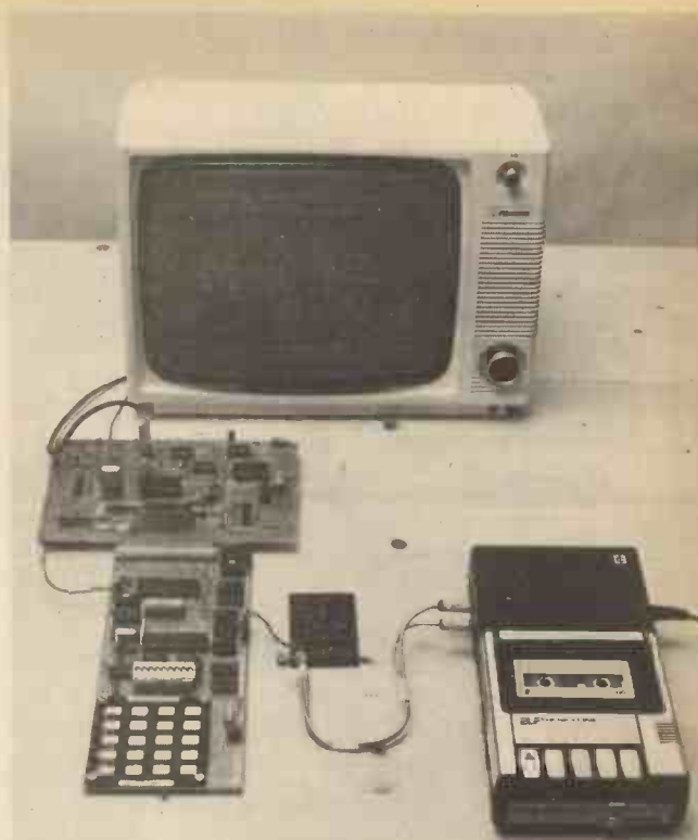
A reasonably sophisticated personal computer resulting from the use of the P.E. VDU with the MK14 and cassette interface
