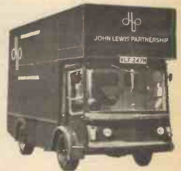
The Crompton Electricars FL85/36 2 tonnes electric delivery van
