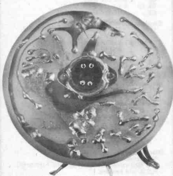
Copper side of board showing mounting of the BT6 (SK1) valveholder base
