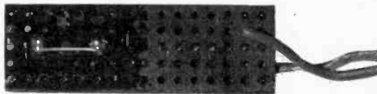
Thermistor mounted on the probe board and covered with an epoxy-resin
