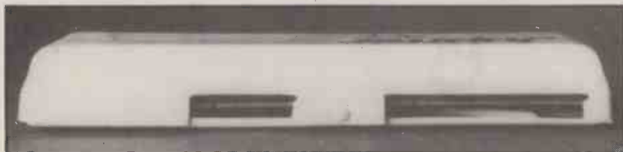
The rear showing the Z-80 bus section and video-output lines reserved for colour.
