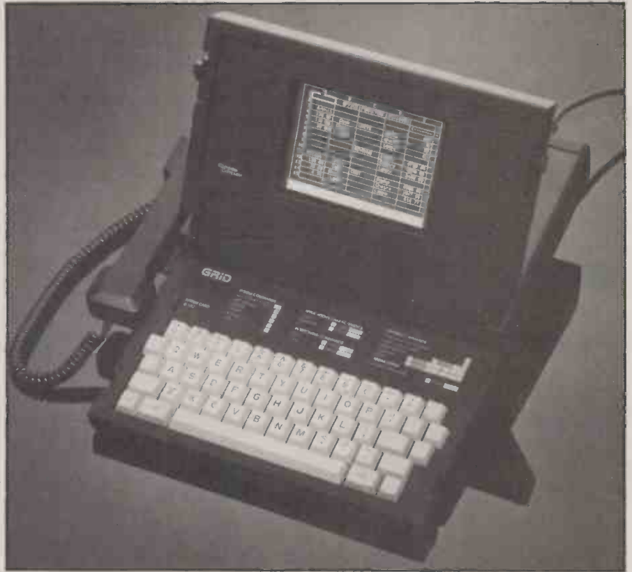
Already available in the U.S., the 10lb. Compass has a 16-bit CPU and built-in Modem.
