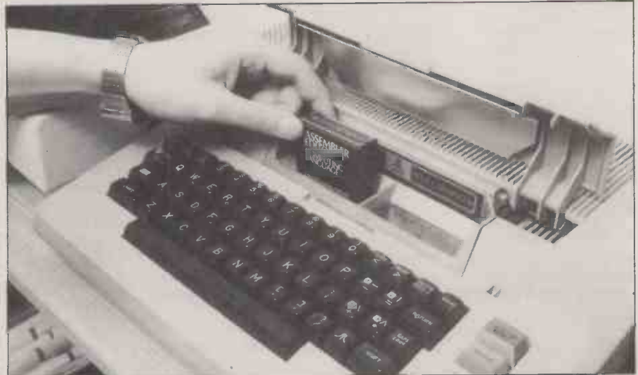
ROM cartridges may be plugged into the slots behind the Atari 800 keyboard.
