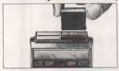
Snap-in more memory. A single module will double the memory available. A quad module adds no fewer than 256 registers at once. Suddenly you've over 1800 lines of memory at your command.
