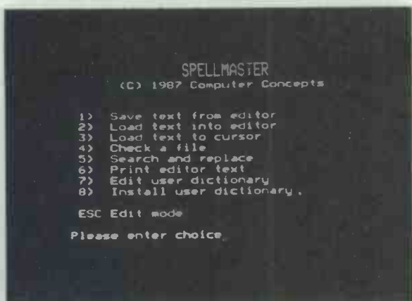
The Spellmaster main menu gives access to a simple text editor, allows modification of user dictionaries, loading and saving of text from the editor, and access to all the 'star' commands
