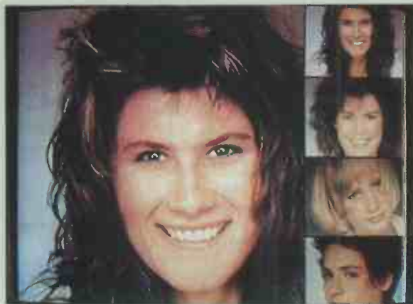
These examples show a set of full-colour photographs input to the computer by means of a video camera. As well as the main picture, up to 15 windows can be displayed holding, among other things, user-generated graphics, images being
