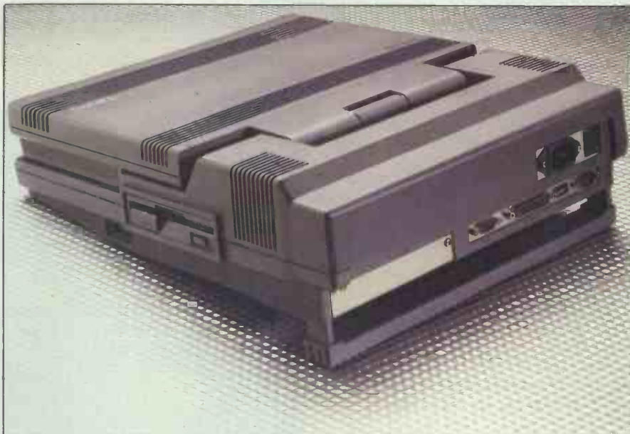
The greater height of the 5100 accommodates the extra memory and video cards. External keyboard and RGB ports allow it to be used purely as a system unit
