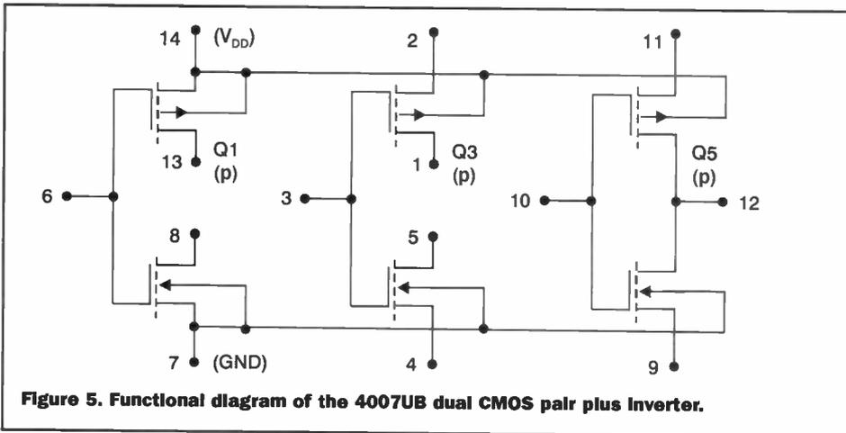
**Figure 5. Functional diagram of the 4007UB dual CMOS pair plus inverter.**
