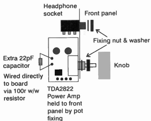
**Figure 16.** The TDA2822 amplifier module is held to the front panel by its volume control. Quite safe - the board is quite light! A 220nF decoupling capacitor wired across the power supply terminals helps to reduce noise from the switch-mode power supply.
