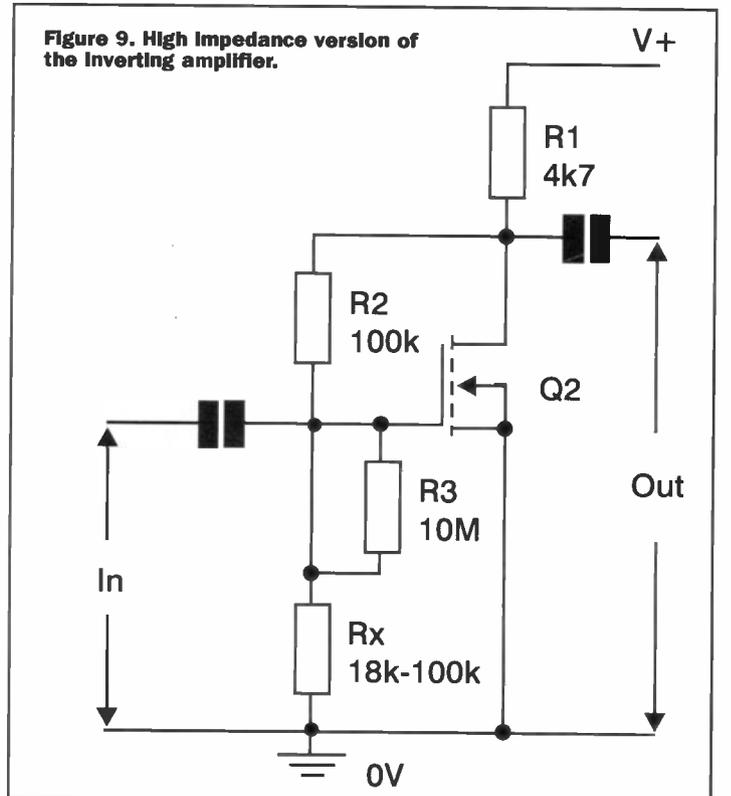
**Figure 9. High Impedance version of the Inverting amplifier.**
