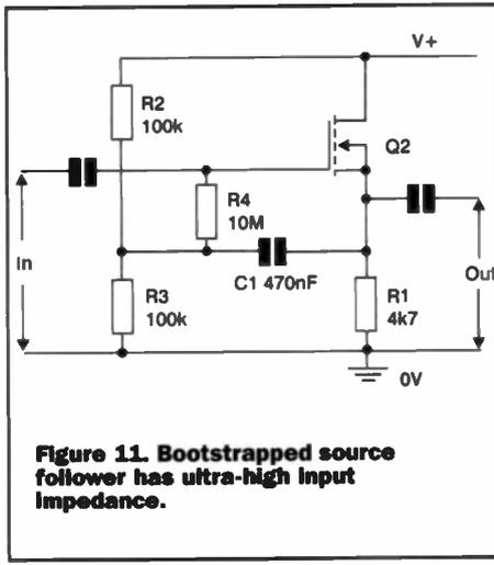
**Figure 11. Bootstrapped source follower has ultra-high input impedance.**
