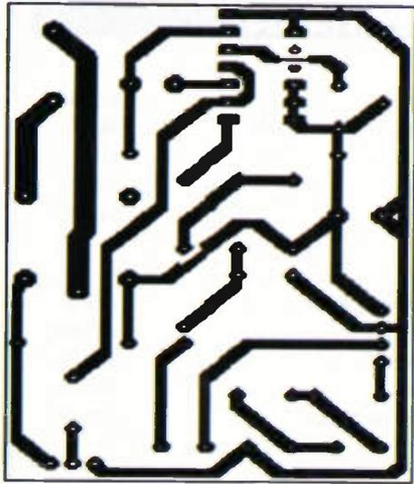
Figure 2. The PCB foil.
