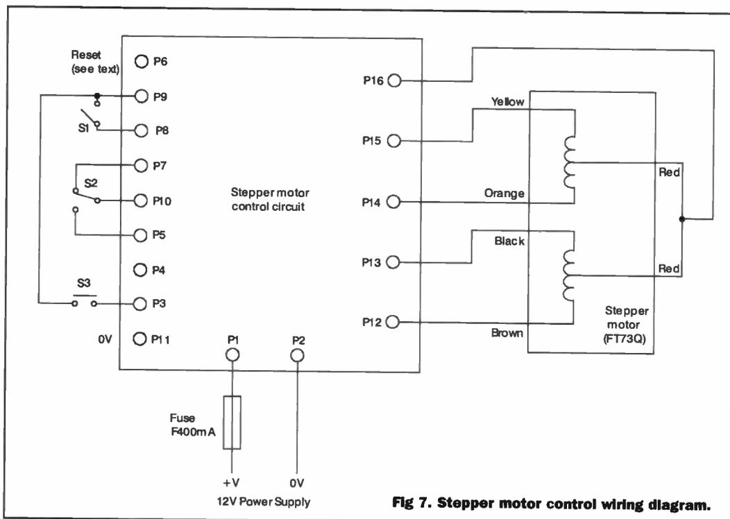
**Fig 7. Stepper motor control wiring diagram.**
