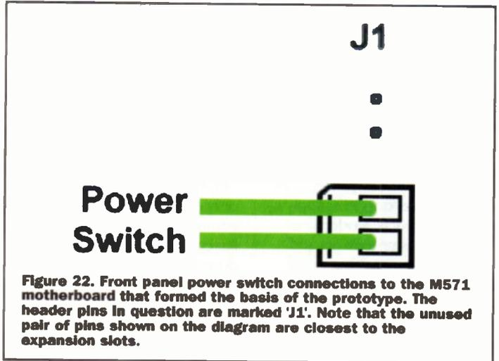
Figure 22. Front panel power switch connections to the M571 motherboard that formed the basis of the prototype. The header pins in question are marked 'J1'. Note that the unused pair of pins shown on the diagram are closest to the expansion slots.
