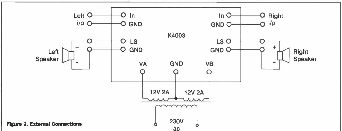
**Figure 2. External Connections**
