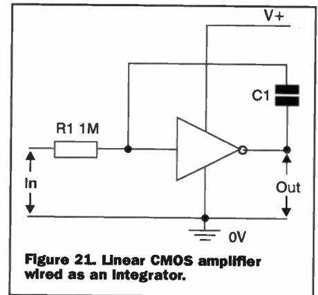
**Figure 21. Linear CMOS amplifier wired as an integrator.**
