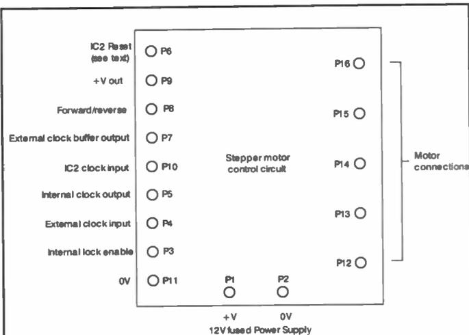
**Fig 8. Stepper motor control terminal designations.**
