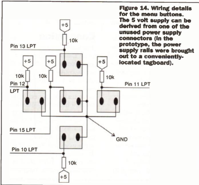
**Figure 14. Wiring details for the menu buttons. The 5 volt supply can be derived from one of the unused power supply connectors (In the prototype, the power supply rails were brought out to a conveniently-located tagboard).**
