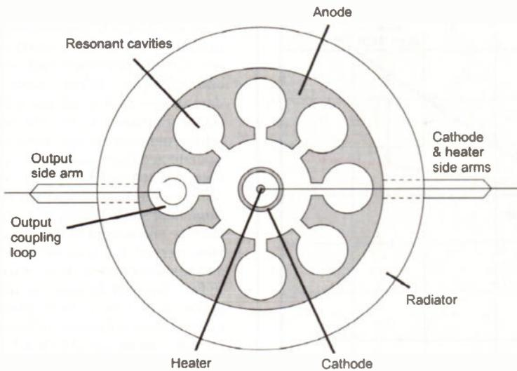
**Figure 39. Typical magnetron structure**
