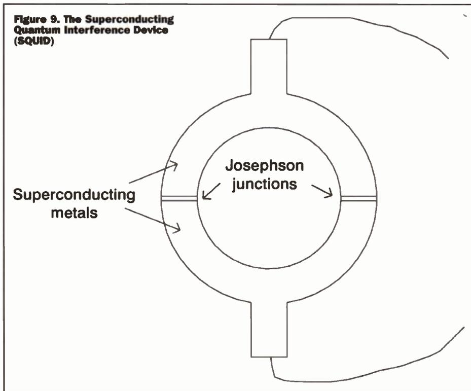
**Figure 9. The Superconducting Quantum Interference Device (SQUID)**
