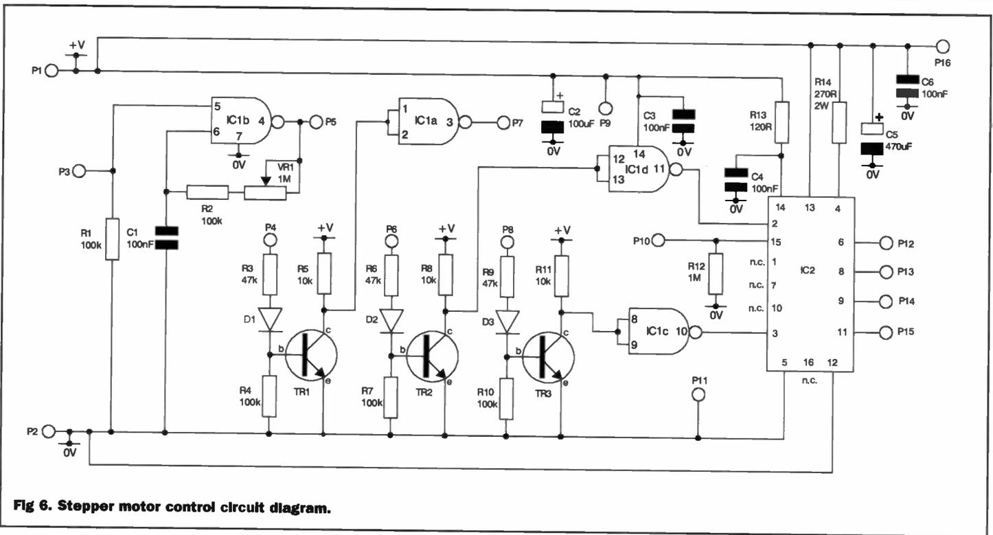
**Fig 6. Stepper motor control circuit diagram.**
