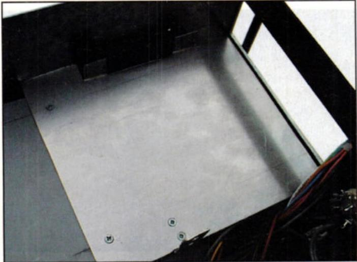
An aluminium plate provides support for the prototype's CD-ROM drive. This plate, which can be seen here, is fitted between the power supply and the front panel.
