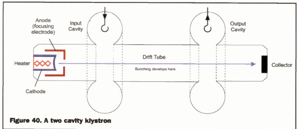
Figure 40. A two cavity klystron
