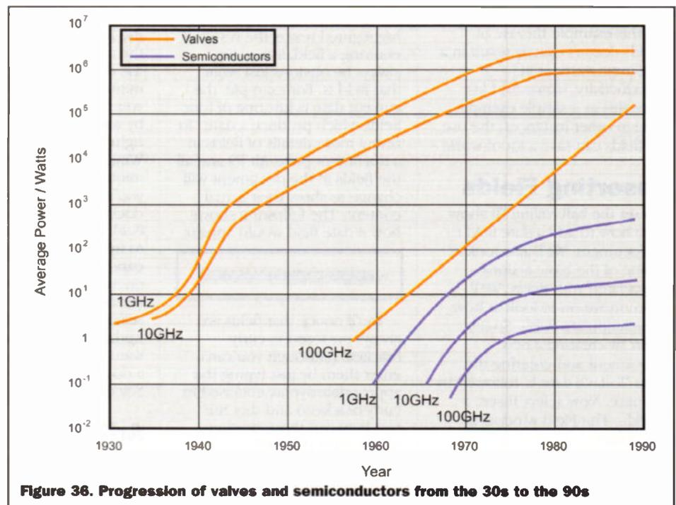
Figure 36. Progression of valves and semiconductors from the 30s to the 90s
