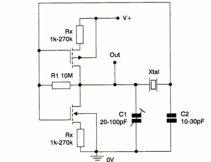
**Figure 23. Micropower version of the crystal oscillator.**
