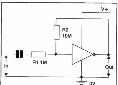
**Figure 19. Linear CMOS amplifier wired as x10 inverting amplifier.**
