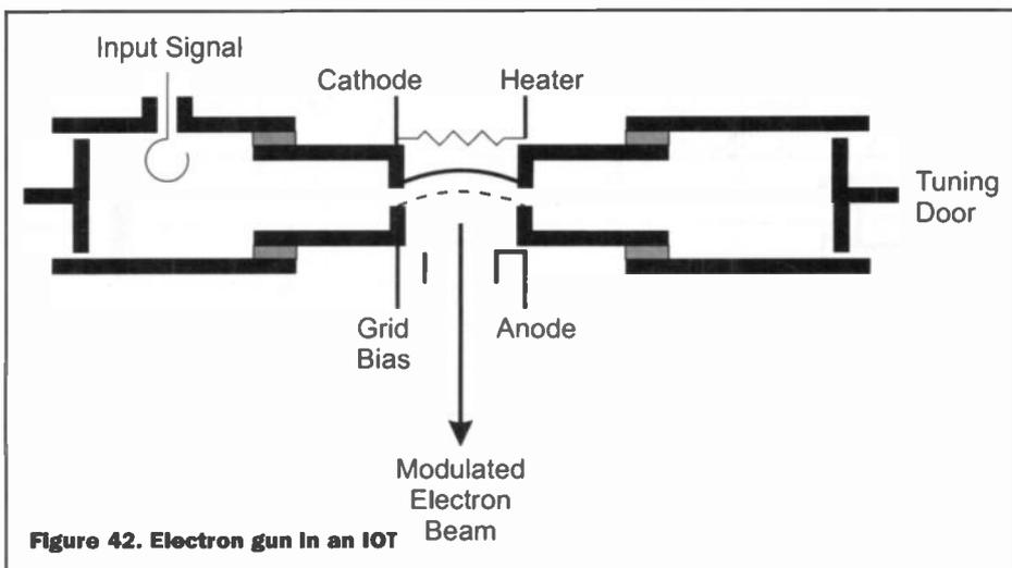
Figure 42. Electron gun in an IOT
