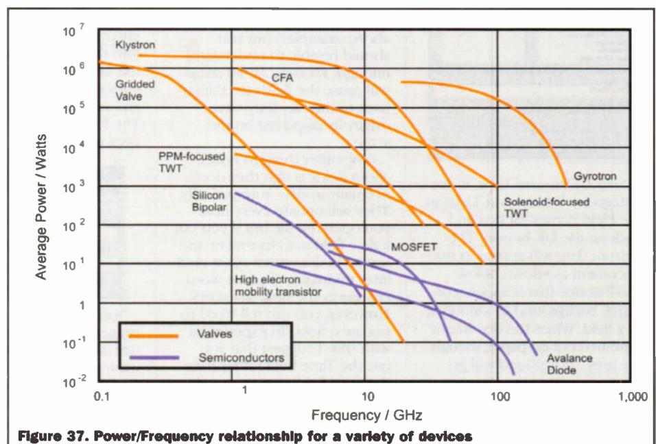
Figure 37. Power/Frequency relationship for a variety of devices
