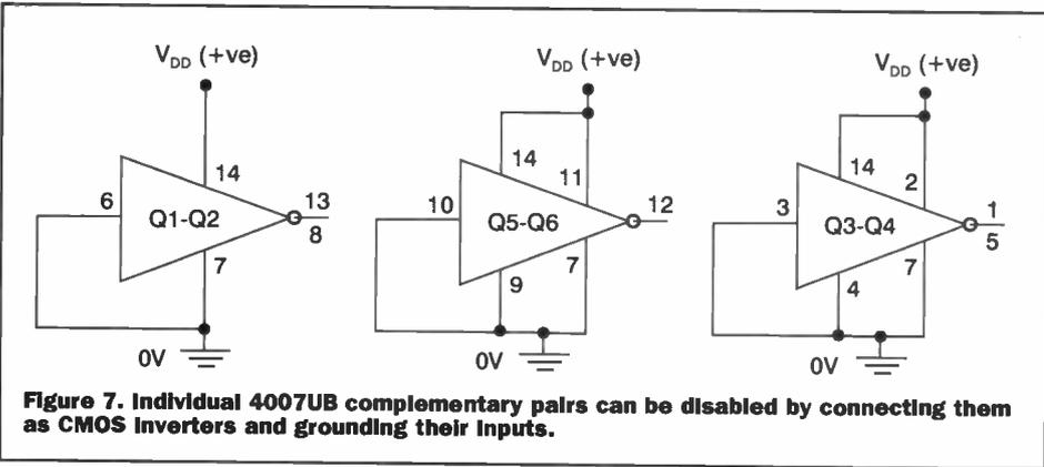
**Figure 7. Individual 4007UB complementary pairs can be disabled by connecting them as CMOS inverters and grounding their inputs.**
