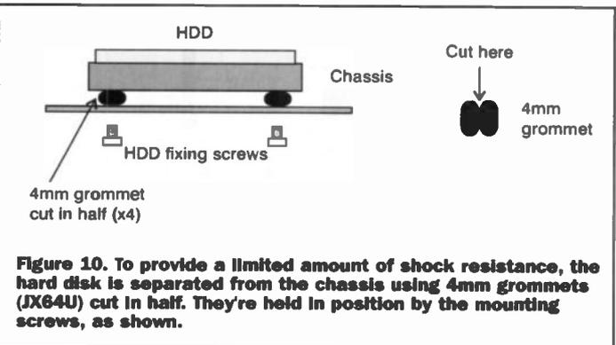
**Figure 10.** To provide a limited amount of shock resistance, the hard disk is separated from the chassis using 4mm grommets (JX64U) cut in half. They're held in position by the mounting screws, as shown.
