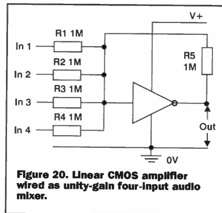
**Figure 20. Linear CMOS amplifier wired as unity-gain four-input audio mixer.**
