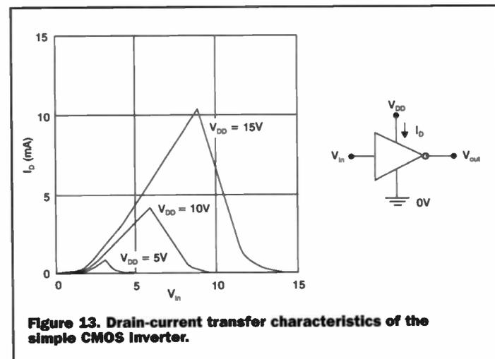
**Figure 13. Drain-current transfer characteristics of the simple CMOS inverter.**
