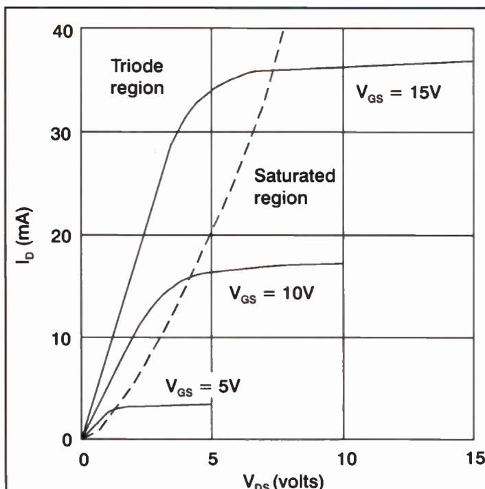
**Figure 3.** Typical transfer characteristics of 4007UB n-channel enhancement-mode MOSFETs.
