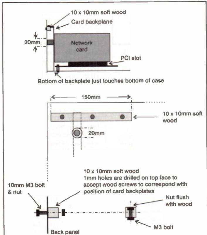
**Figure 12.** Details of card mounting, showing position of wooden dowelling used to secure any expansion cards (sound/network, etc.)
