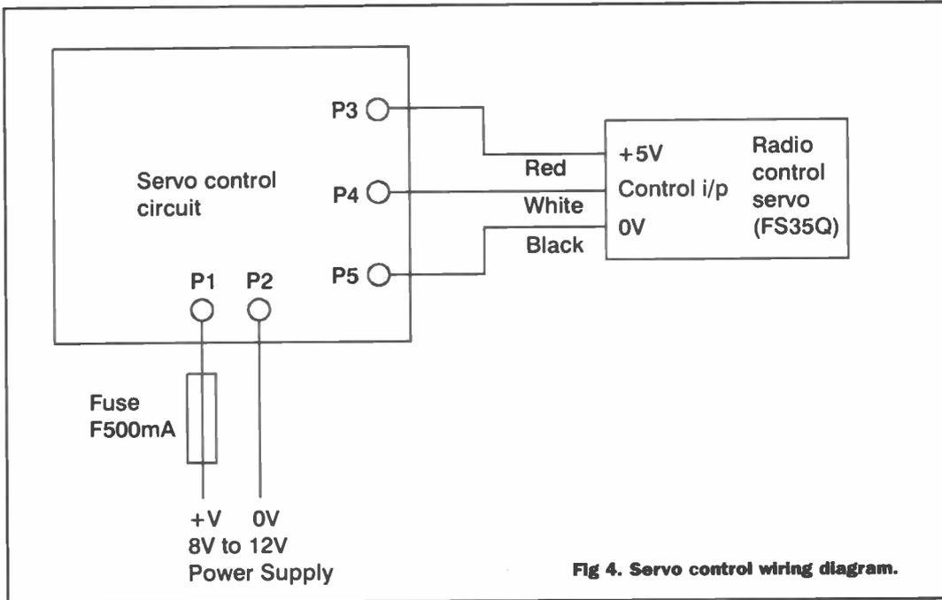
Fig 4. Servo control wiring diagram.
