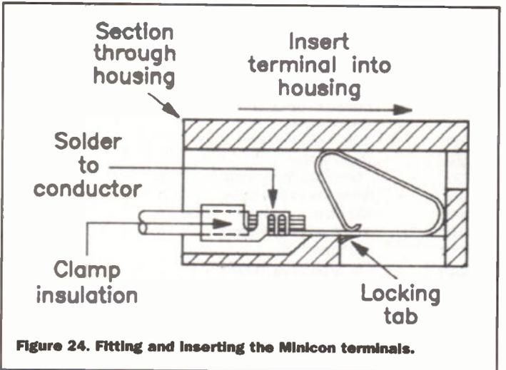
Figure 24. Fitting and inserting the Minicon terminals.
