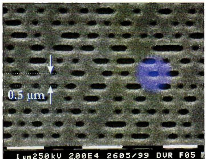
Figure 1a/b. The reduction in pit and laser spot size
