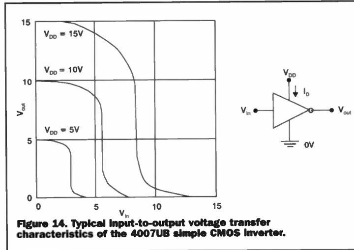
**Figure 14. Typical input-to-output voltage transfer characteristics of the 4007UB simple CMOS inverter.**
