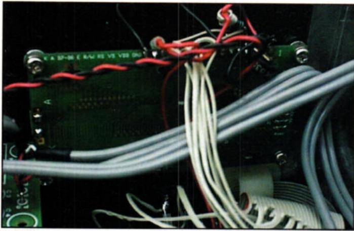
Close-up view of the display and keypad wiring. A self-adhesive cable tie (VK43W) clips the ribbon cable to the front panel.
