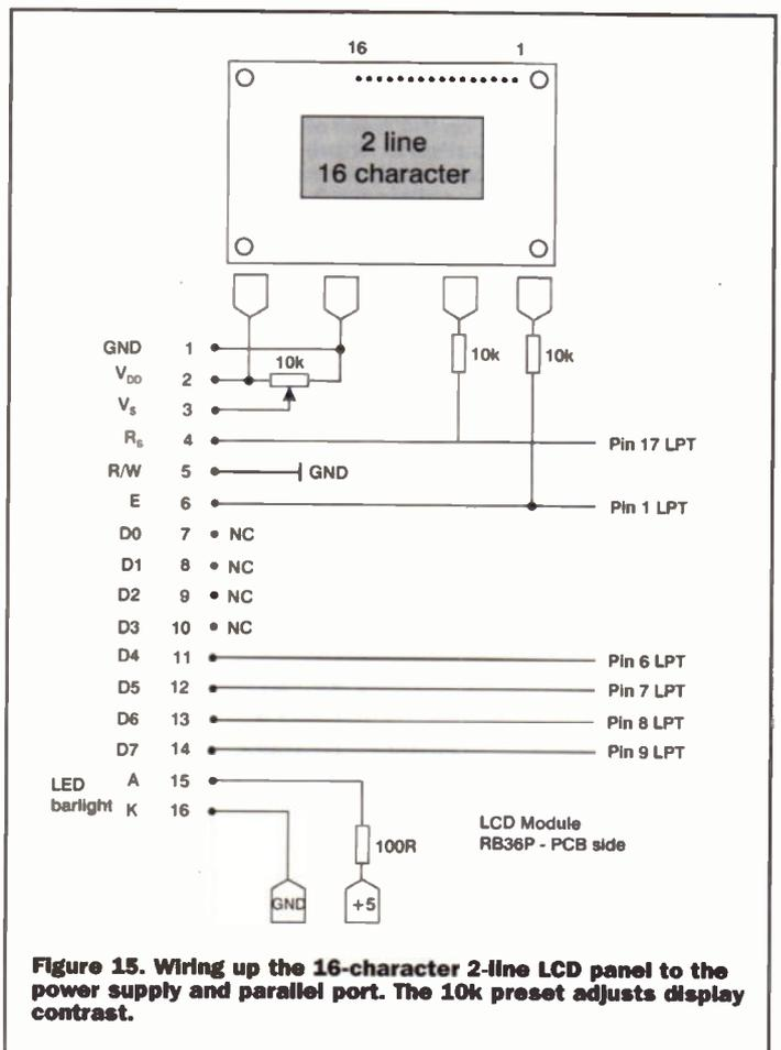
**Figure 15. Wiring up the 16-character 2-line LCD panel to the power supply and parallel port. The 10k preset adjusts display contrast.**
