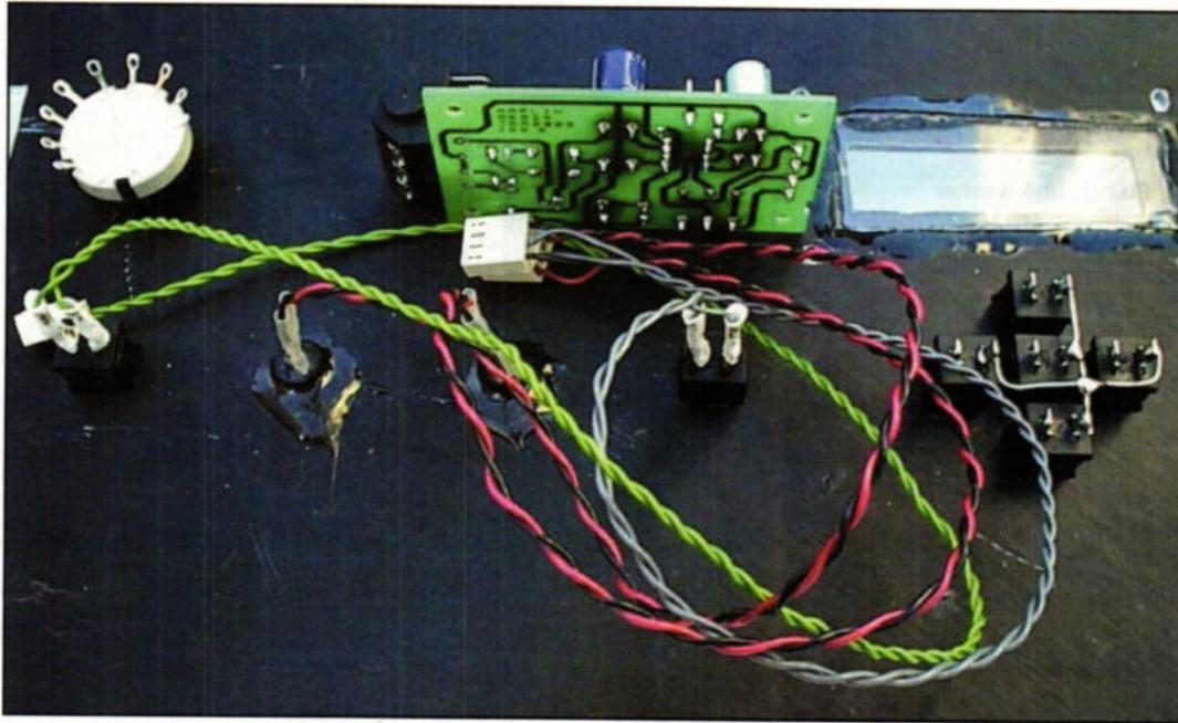
At the time this photo was taken, the front panel was in the process of being fitted out. Note the clear plastic that has been epoxied to the display cut-out. This sheet, which was cut from an old cassette tape, has been provided to protect the LCD screen.
