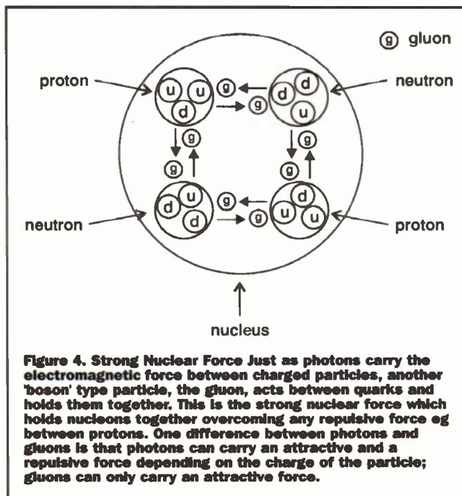
**Figure 4. Strong Nuclear Force Just as photons carry the electromagnetic force between charged particles, another 'boson' type particle, the gluon, acts between quarks and holds them together. This is the strong nuclear force which holds nucleons together overcoming any repulsive force eg between protons. One difference between photons and gluons is that photons can carry an attractive and a repulsive force depending on the charge of the particle; gluons can only carry an attractive force.**
