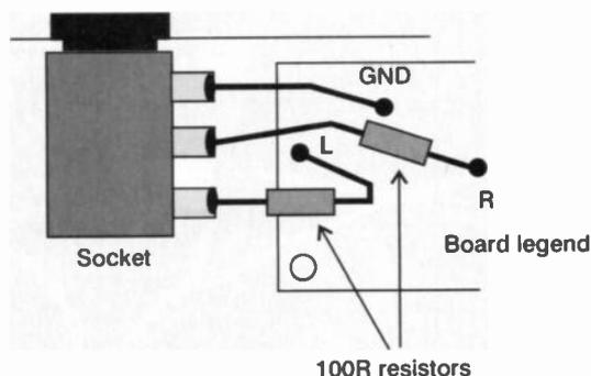
**Figure 17.** How to wire up the 6.3mm headphone socket - the drawing is specific to the 3.5mm headphone socket of Maplin board legend. Note the use of 100Ω resistors - these limit volume, but also attenuate noise.
