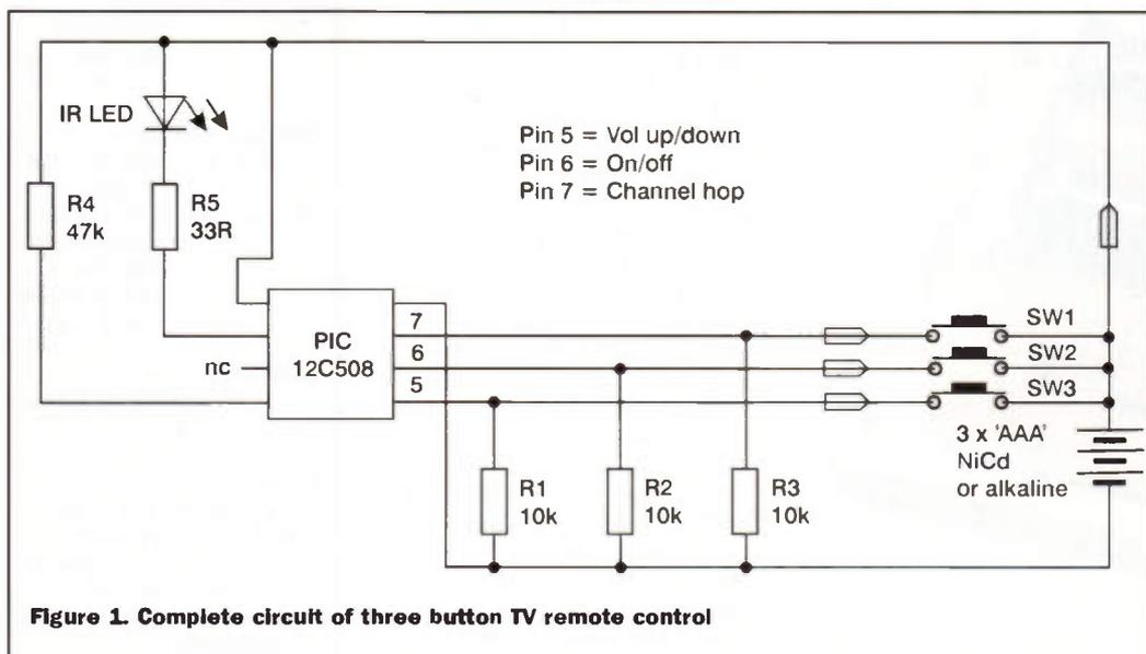
Figure 1. Complete circuit of three button TV remote control
