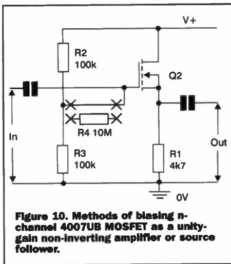
**Figure 10. Methods of biasing n-channel 4007UB MOSFET as a unity-gain non-inverting amplifier or source follower.**
