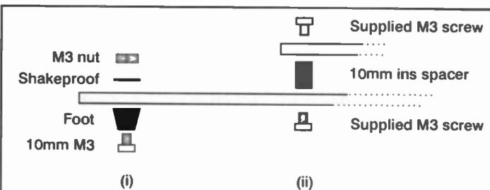
**Figure 8.** How to fit the feet (FW19V) and 10mm motherboard spacers (FS36P).
