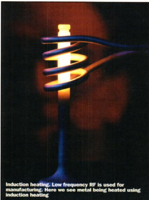
Induction heating. Low frequency RF is used for manufacturing. Here we see metal being heated using induction heating
