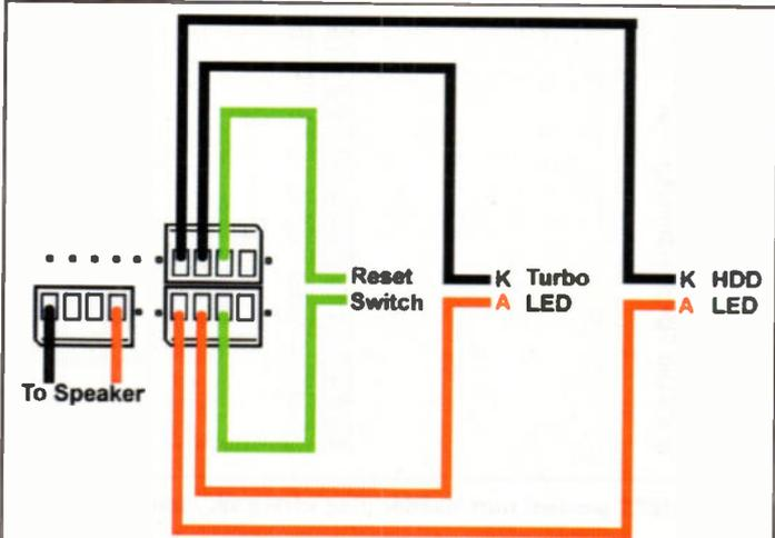
Figure 21. Reset switch, speaker and LED connections to the M571 motherboard that formed the basis of the prototype. The header pins are located towards the bottom-left of the board. The lower row of pins, as shown in the diagram, are nearest the board edge.
