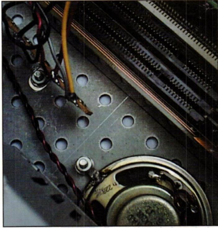
Here's a close-up view of the tag-strip, which is used to provide a convenient access point for the +5/+12V supply rails. These voltages, which are sourced from one of the power supply's unused disk drive connectors, are needed to power the display and headphone amplifier. The speaker, and its solder-tag mounting arrangement, can also be seen.
