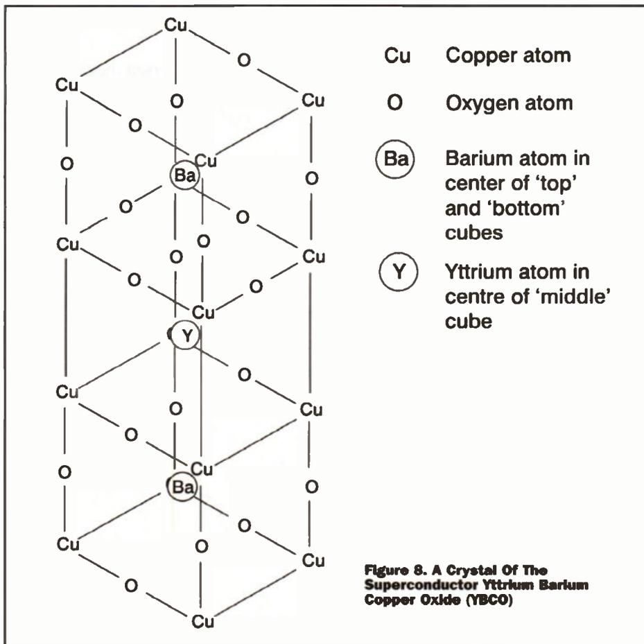
**Figure 8. A Crystal Of The Superconductor Yttrium Barium Copper Oxide (YBCO)**
