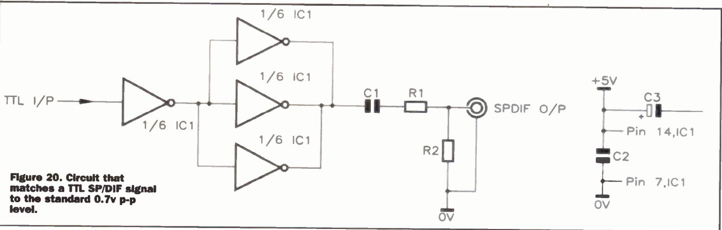
Figure 20. Circuit that matches a TTL SP/DIF signal to the standard 0.7v p-p level.
