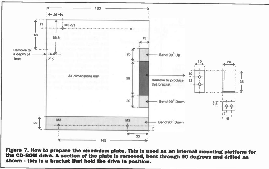
**Figure 7.** How to prepare the aluminium plate. This is used as an internal mounting platform for the CD-ROM drive. A section of the plate is removed, bent through 90 degrees and drilled as shown - this is a bracket that hold the drive in position.
