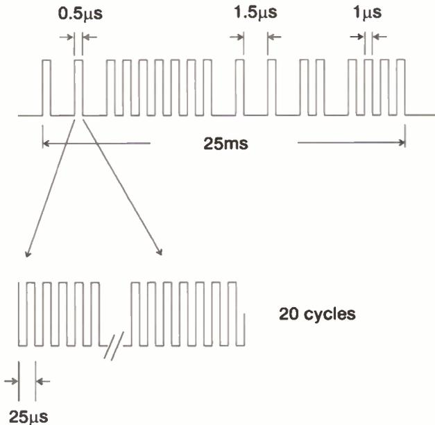
Figure 2. The code for ON/OFF for a JVC television
