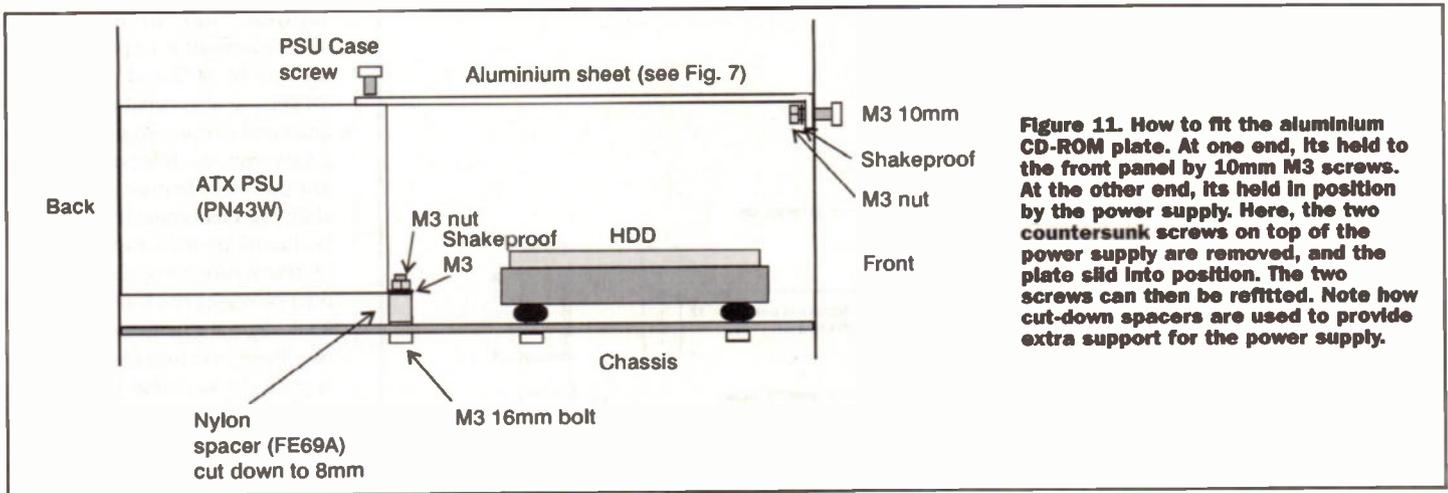
**Figure 11.** How to fit the aluminium CD-ROM plate. At one end, its held to the front panel by 10mm M3 screws. At the other end, its held in position by the power supply. Here, the two countersunk screws on top of the power supply are removed, and the plate slid into position. The two screws can then be refitted. Note how cut-down spacers are used to provide extra support for the power supply.
