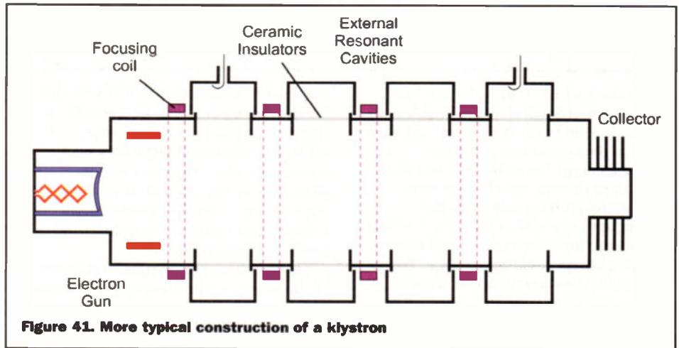
Figure 41. More typical construction of a klystron
