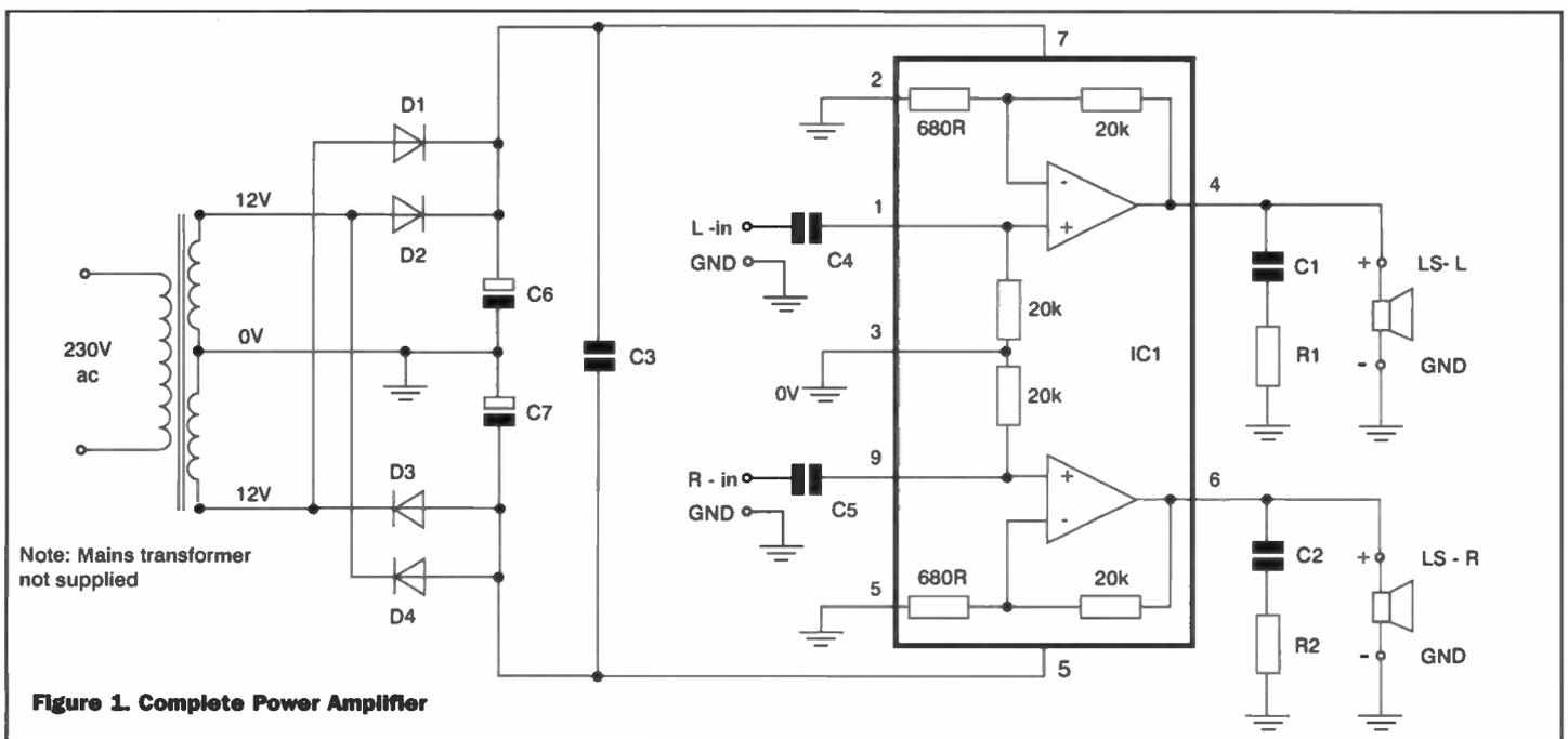
**Figure 1. Complete Power Amplifier**
