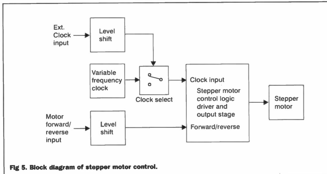
Fig 5. Block diagram of stepper motor control.
