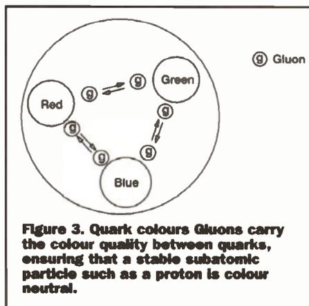
**Figure 3. Quark colours Gluons carry the colour quality between quarks, ensuring that a stable subatomic particle such as a proton is colour neutral.**
