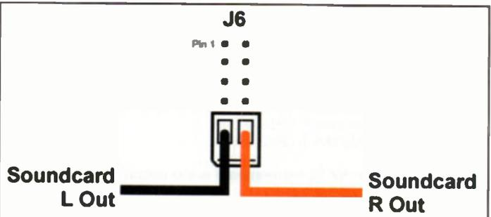
Figure 23. This diagram indicates where the stereo audio outputs are located on the M571 motherboard that formed the basis of the prototype. The header pins are marked 'J6', and can be found towards the top-left of the board.
