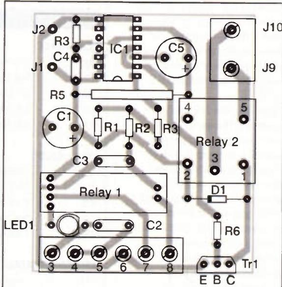
Figure 3. Component overlay.
