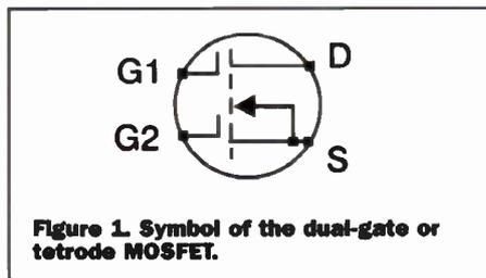
**Figure 1.** Symbol of the dual-gate or tetrode MOSFET.
