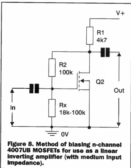
**Figure 8. Method of biasing n-channel 4007UB MOSFETs for use as a linear inverting amplifier (with medium input impedance).**
