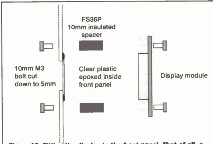
**Figure 13.** Fitting the display to the front panel. First of all, a piece of clear plastic is epoxied to the front panel. The purpose of this plastic, which could be obtained from an old cassette or CD case, is to protect the display. Note that the M3 screws supplied with the spacers are not long enough to penetrate the front panel - you will have to obtain 10mm M3 screws and cut those down to 5mm.
