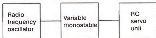
Fig 1. Simple pulse generator block diagram.
