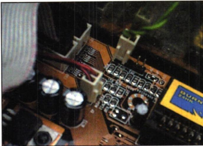
**Close-up view of JP1 - the M571 motherboard's power switch - and the Minicon connector that's attached to it (refer to Figure 22). The other connector supplies power to the microprocessor's fan.**
