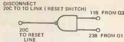
4.9 Automatic resetting on a count of ten. This lets us use binary counters for counting denary scale (BCD, which is binary coded decimal)
