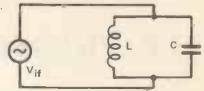
Figure 6. Parallel resonant circuit
