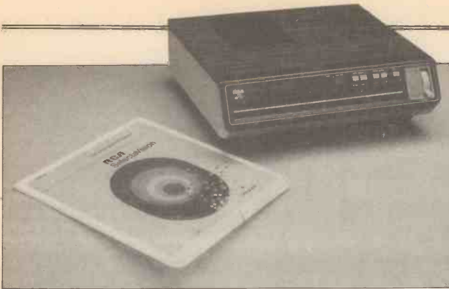
Figure 5. RCA's SelectaVision player with CED disc alongside
