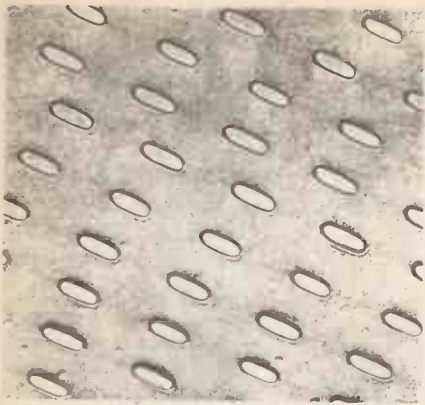
Figure 2. Formation of pits on a VLP disc: a) electron microscope view of disc surface
