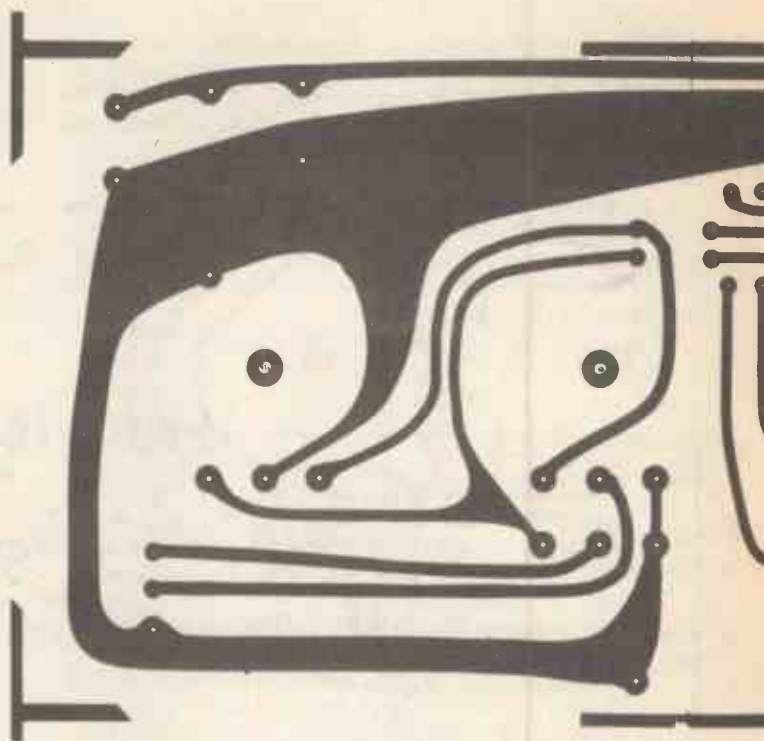
Fig. 2. PCB for the pre-amp.
