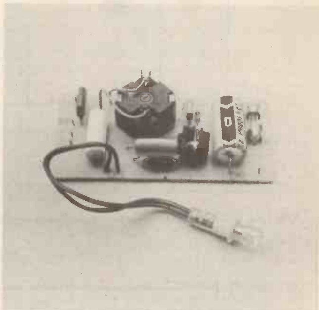
This miniature power-house will take the tarnish off your tracks. The ferrite-cored transformer makes an efficient high voltage generator that will really dust off the debris.
