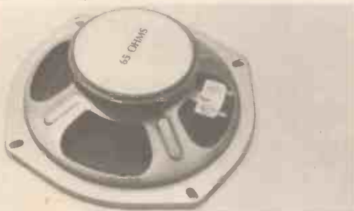
Fig. 4.8. The appearance of the loudspeaker; a high-resistance type is essential.
