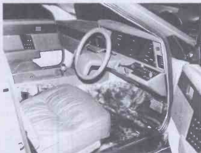
Interior shot of the Aston Martin Lagonda instrument panel. Most of the secondary controls are operated by the labelled touch pads on the console.
