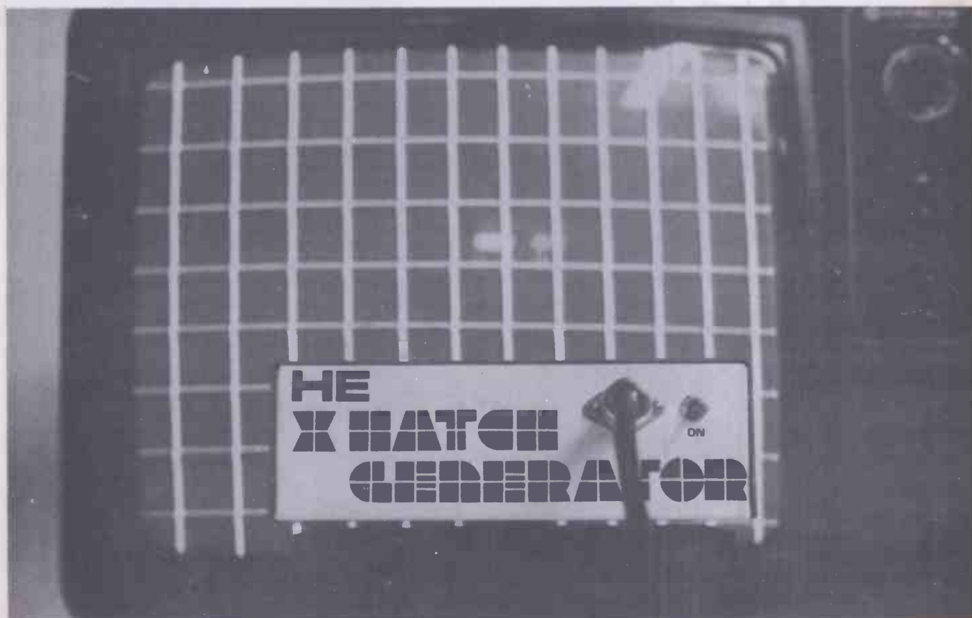
The HE Crosshatch Generator connected up to a TV set. Convergence errors are most noticeable at the corners of the picture.
