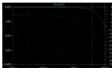
**A 10k volume control set half way offers maximum source impedance. Capacitance seen by the output slider will roll down treble. Diagram and analysis by LTSpice.**
