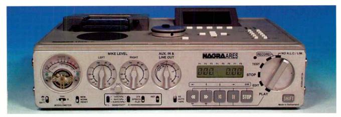
The fascia carries all the major controls like the twin microphone level and single Line In and Out potentiometers. The 'Modulometer' to the far left aids in the setting of the record level, while the rotary switch to the far left controls operational modes like Play and Record.
