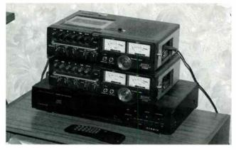
Cassette replay and recording comes courtesy of a pair of Sony TC158SDs.
