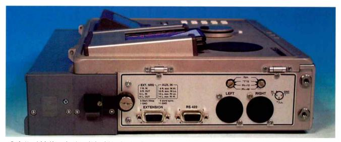
On the Nagra's left side panel are located left and right microphone inputs, the 15-pin line-level input (far left) and the RS 422 socket which allows connection to a PC.
