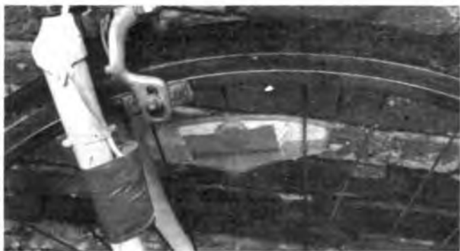
The magnetic field sensor taped to the bike fork and the magnet glued and taped to a plastic reflective plate attached to the wheel spokes.
