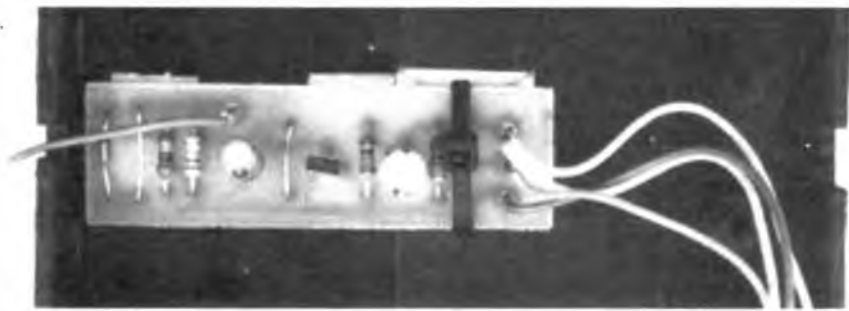
A cable tie with a self-adhesive base secures the Trigger p.c.b. to the case lid. There are various component use options available which is why this board appears to differ from the detail in Fig. 4.
