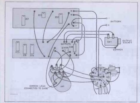
Fig. 5. Interwiring to the boards, VR1, JK1 and switch S1.
