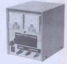
A superb design giving 0-25V and 0-2.5A. Twin par meters indicate Voltage and Current. Voltage is va able from zero to 25V.
