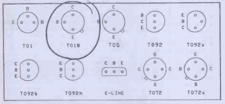
Fig. 2.12. Example of transistor base identification chart. (Diagram taken from *Electronic Hobbyists Handbook* published by Babani)
