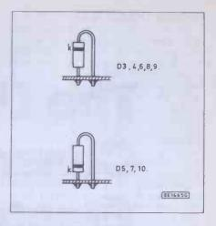
Fig. 4. Polarity guide for mounting the diodes on the p.c.b.
