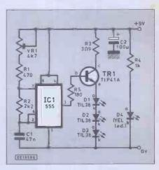
Fig. 2. Transmitter circuit diagram.
