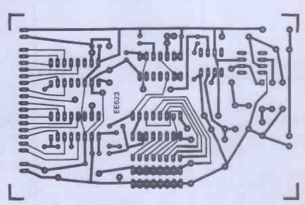
Fig. 4. Main p.c.b. for the I.R. Object Counter.
