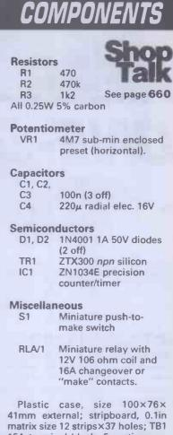
41mm external; stripboard, 0.1in matrix size 12 stripsx37 holes; TB1 15A terminal block-5 sections required; FS1 20mm chassis fuseholder with 1A fuse to fit; 14-pin d.i.l. i.c. socket; 3A auto-type wire; 7A auto-type wire; auto-type connectors; small fixings; etc.
