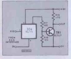
Fig. 2: The Digital Isolation circuit diagram
