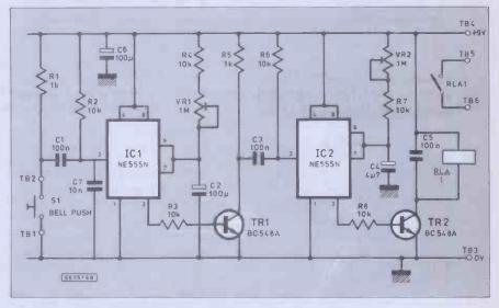
Fig. 1. Circuit for the Doorbell Delay
