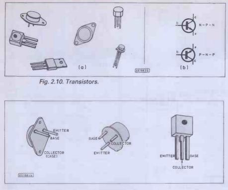
Fig. 2.11. Typical transistor leadouts.
