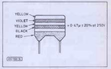
Fig. 2.8. Example of capacitor colour coding.
