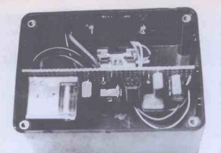
leaving some slack. Adjust preset VR1 sliding contact fully clockwise then anticlockwise by one sixteenth turn approximately. Insert the fuse. Place IC1 carefully into its socket with the correct orientation and slide the circuit panel into position.
