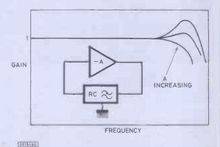
Fig. 2. When an RC lowpass with three or more sections is connected as a feedback path in an inverting amplifier the frequency response becomes very dependent on the gain when the phase shift of the network is close to 180°. Adding the input signal to the feedback is arranged for by resistors R1 and R2. At very low frequencies the gain is mainly defined by these resistances, which form a negative feedback network.
