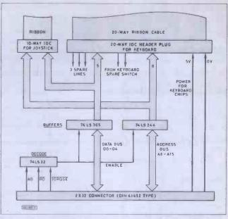
Fig. 3 (above). Details of suggested keyboard interface.
