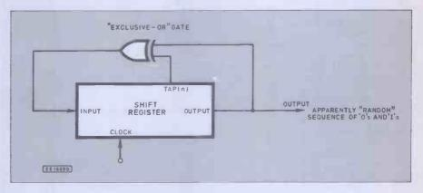
Fig. 1. Simplified digital noise generator using a shift register.
