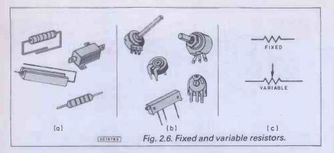
when selecting one for use: the actual resistance value in ohms (symbol  $\Omega$  ) and the tolerance rating which is the guaranteed degree of accuracy to which the resistor is manufactured.
