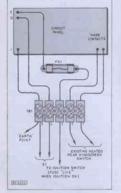
Fig. 2. P.C.B. layout and wiring. Fig. 3 (left). Internal wiring and car connections.
