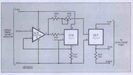
Fig. 3. The Analogue Isolation circuit diagram
