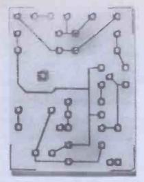
Fig. 2.1 (above). The underside of a p.c.b. before the components are inserted.
