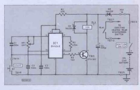
Fig. 1. Circuit diagram of the one-shot timer.
