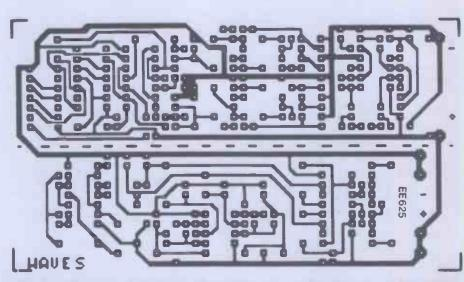
Fig. 3. printed circuit board component layout and full size copper foil master pattern. This board is cut in half to form two boards, if using the case specified.
