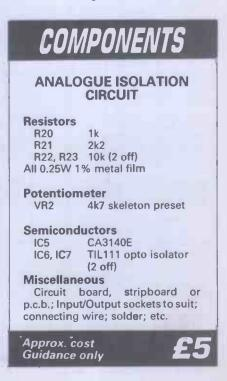
In practice it is not possible to obtain perfectly matched opto-isolators. Preset VR2 can be adjusted to compensate for moderate differences in the efficiencies of the two isolators so that approximately unity voltage gain is obtained, but a certain amount of distortion will have to be tolerated.
