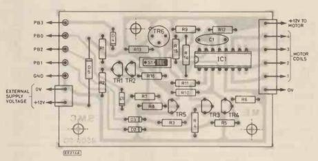
Fig. 6. Component layout for the Stepper Motor Interface.
