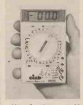
Nine functions and 29 measuring ranges are available from the multimeter. The resistance ranges are from 200 ohm to 20 megohm, in six switched ranges. The a.c. and d.c. amps ranges cover from 200µ to 200mA, in four ranges. There is also a position for 10A measurement.
