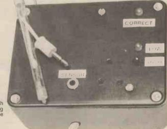
The encased unit with the temperature-sensing thermistor visible at the end of the glass rod.
