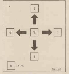
Fig. 1. Relationship between joystick functions and keyboard.
