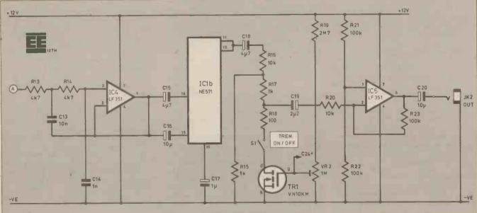
Fig. 2. Main circuit diagram. This is split in two parts-points "A" and the supply lines connect.
