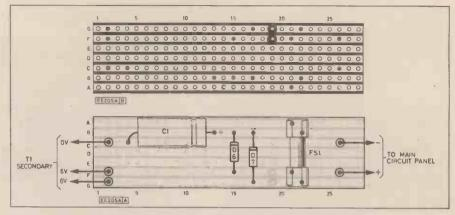
Fig. 5. Component layout for the mains-power circuit.
