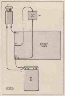
Fig. 4. Connections for battery operation.
