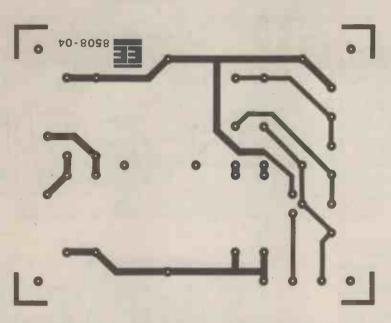
Fig. 2. Printed circuit board (actual size) for the Drill Control Unit. This board is available from the *EE PCB Service*, quote order code: 8508-04.
