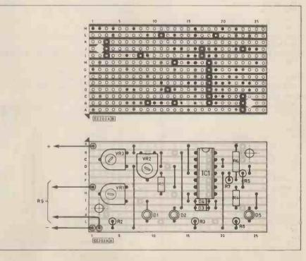
Fig. 3. Component layout and stripboard drilling details.
