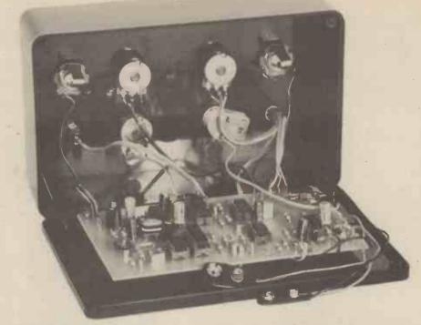
the circuit. SI can be used to switch out TR1 and remove the tremolo effect.
