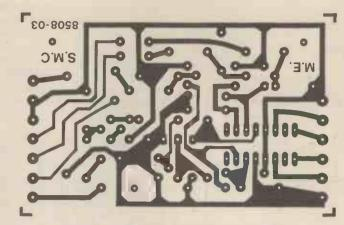
Fig. 5. P.c.b. design for the Stepper Motor Interface
