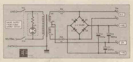
Fig. 11. Complete circuit diagram of the Low Cost PSU.
