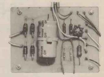
size. The tie-wrap passes around the capacitor and through holes in the p.c.b. on each side. Also, the transistor TR1 was fitted with a push-on T0-18 heatsink which will aid dissipation when the transistor is conducting.
