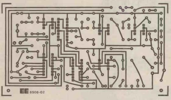
Fig. 4. Printed circuit board layout and wiring.
