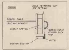
Fig. 7. IDC socket assembly.
