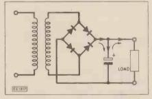
Fig. 9. The capacitor is supplied with energy.
