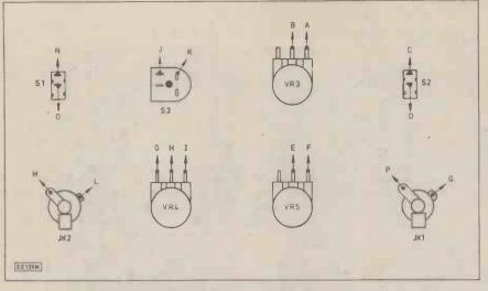
Fig. 5. Front panel wiring.
