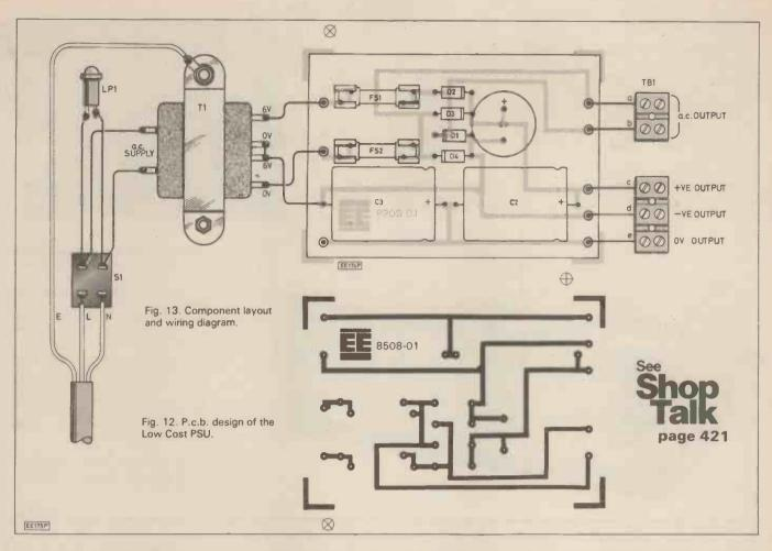
A bridge rectifier, D1-D4 is used to give full wave rectification which provides a positive and negative voltage with respect to the centre tap. The capacitor, C1 smooths the supply to provide a steady d.c. output. Capacitors, C2 and C3 also smooth the supply and also help prevent the positive and negative voltages drifting with respect to OV.
