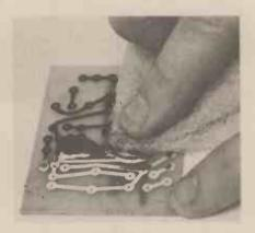
and the process is very similar to that used when drawing the board, with the exception that mistakes, modifications and improvements can be made much more easily by removing the lines and pads from the acetate by gentle scraping.
